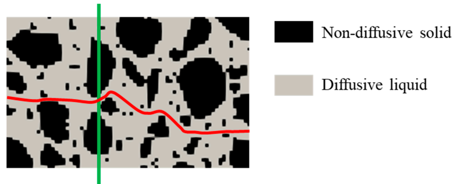
Figure 1. Schematic illustration of the effects of tortuosity and reduced cross-section area on diffusive flux. The black area and grey area refer to the non-diffusive and diffusive parts in cementitious materials. The red line represents a tortuous diffusive path. The green line represents a cross-section with a reduced pore solution area.
