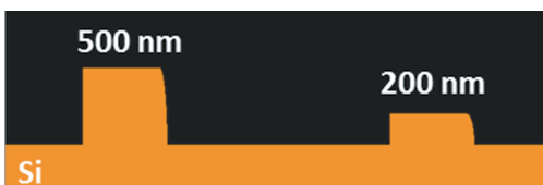
Figure 7.6: Cross-section of lines of 500 and 200 nm in height. The top and the bottom widths of the lines are 500 nm, resp. 550 nm. The pitch is \approx 2\ \mu\text{m} . The left sidewalls of the structures are sharp vertical edges. The right edges are rounded and the side-walls follow the curvature of the edge.
