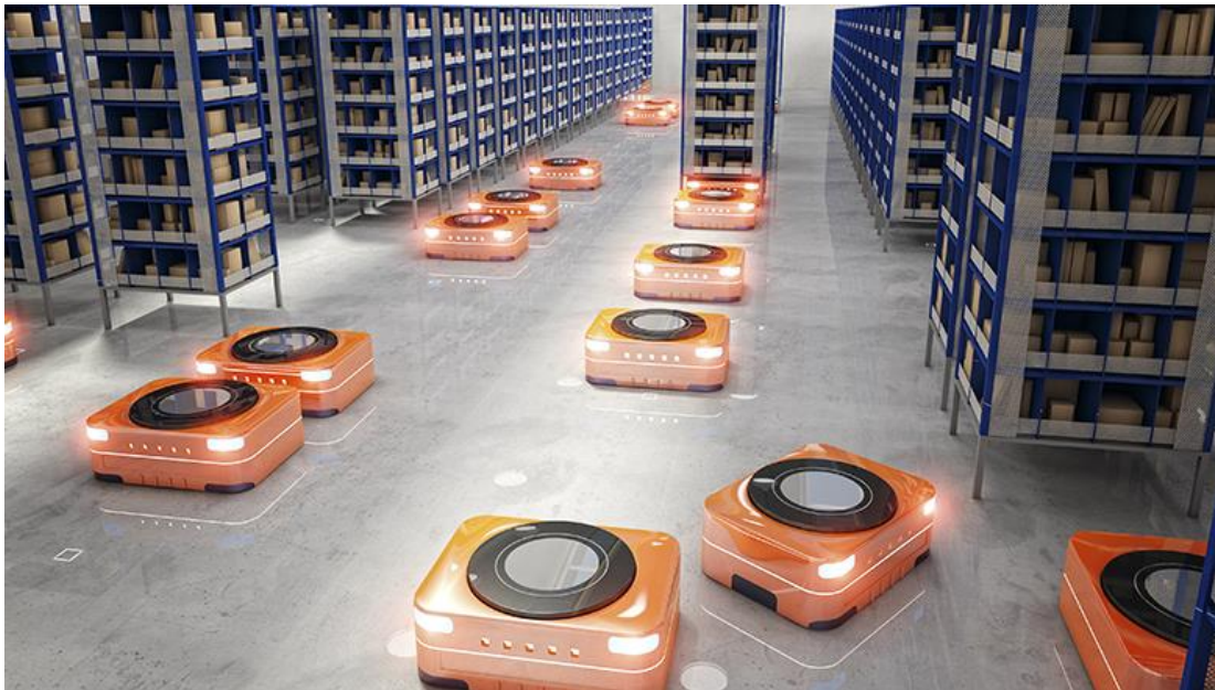
Figure 3 Representation of free ranging AGVs
