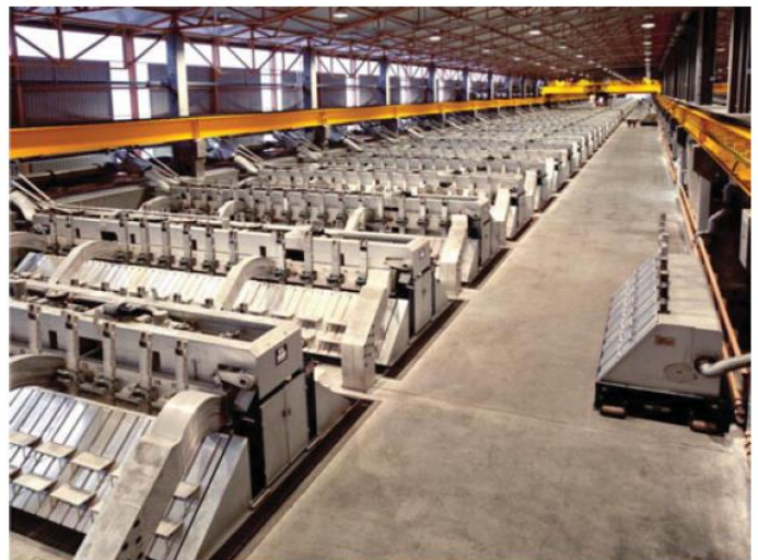
Fig. 5. Modern aluminium potroom [23]
