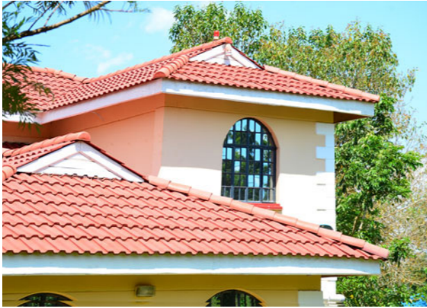
Figure 12: Roof tiles made of local waste plastic in Kenia (EcoBlocks & Tiles, 2019)
