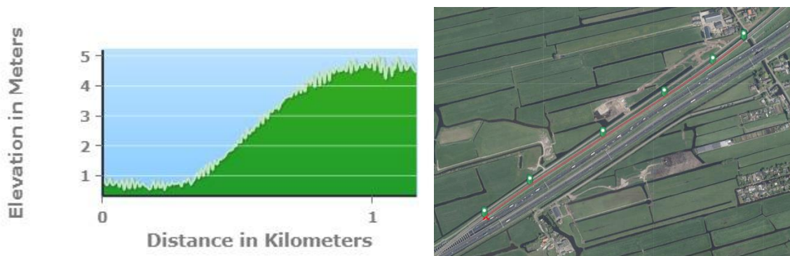
Figure 7 Height profile of the embankment over the distance at the case study (AHN (Actueel Hoogtebestand Nederland))
