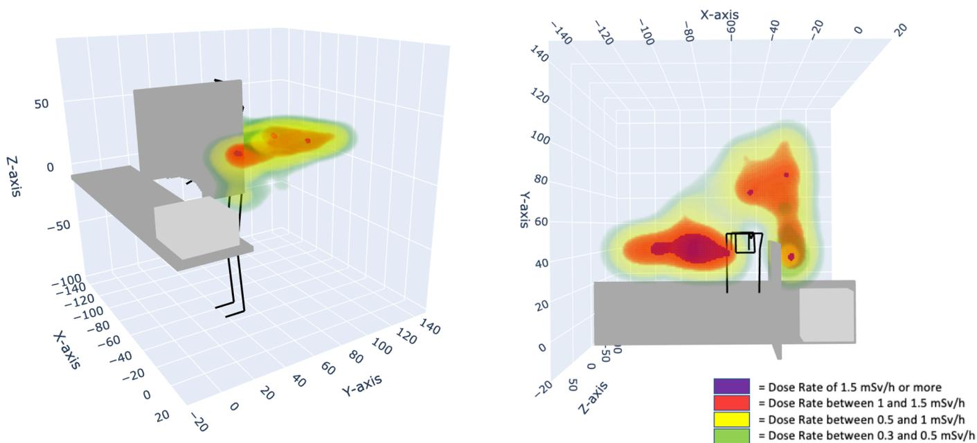
Figure 40: Interpolated visualisation of the data with a lead screen. 40° tilted orientation of the C-arm, Fluoroscopy mode
