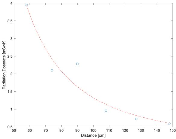
Figure 24: 40° tilted orientation C-arm, Acquisition mode, With lead screen (measurements 105 cm above the ground)
