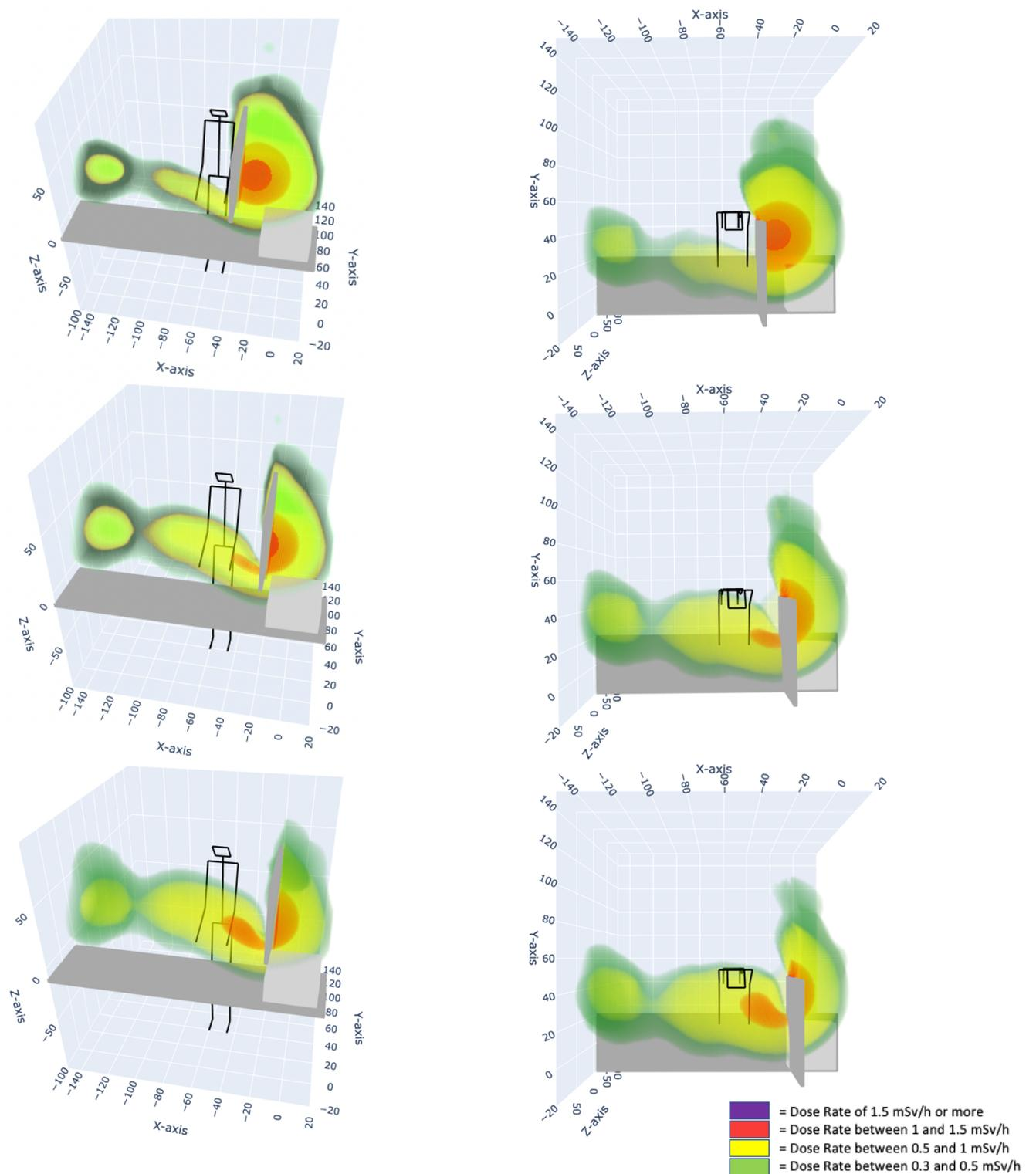
Figure 45: Estimated scatter patterns for three different lead screen positions with an AP orientation of the C-arm. Top: Lead screen positioned 20 cm from the edge of the phantom. Middle: Lead screen positioned 5 cm from the edge of the phantom. Bottom: Lead screen positioned 0 cm from the edge of the phantom.
