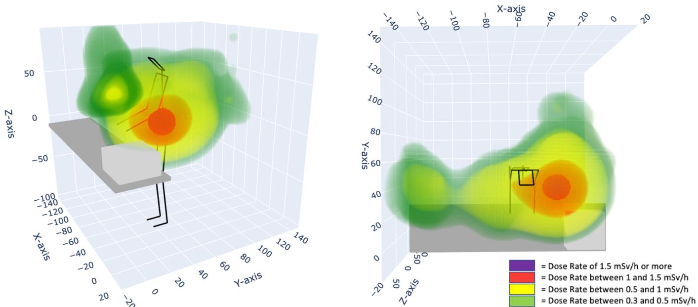
Figure 33: Interpolated visualisation of the data without a lead screen. AP orientation of the C-arm, Acquisition mode
