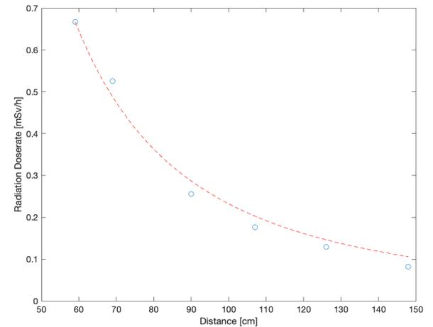
Figure 19: 40° tilted orientation C-arm, Fluoroscopy mode, No lead screen (measurements 105 cm above the ground)
