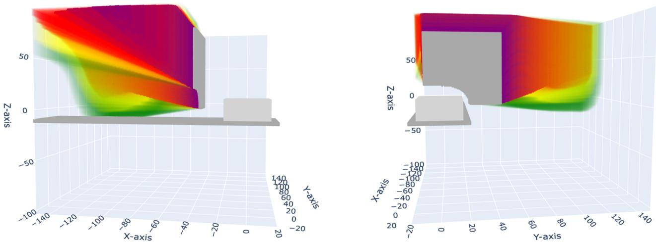
Figure 9: Visualization of the attenuation of the shield. Purple: Attenuation between 75 and 100%, Red: Attenuation between 50 and 75%, Yellow: Attenuation between 25 and 50%, Green: Attenuation between 10 and 25%
