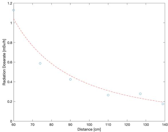
Figure 18: AP orientation C-arm, Acquisition mode, No lead screen (measurements 105 cm above the ground)
