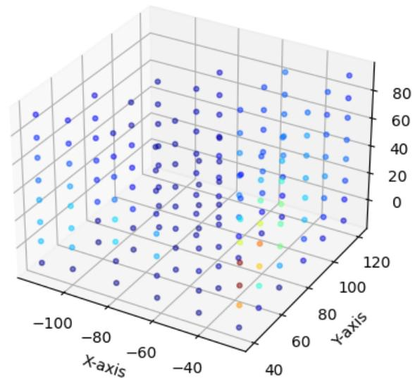
Figure 26: Measurement points; AP orientation, Acquisition mode, With lead screen. The colour of the dots are dependent on the Doserate value, where dark blue is low and dark red is high.
