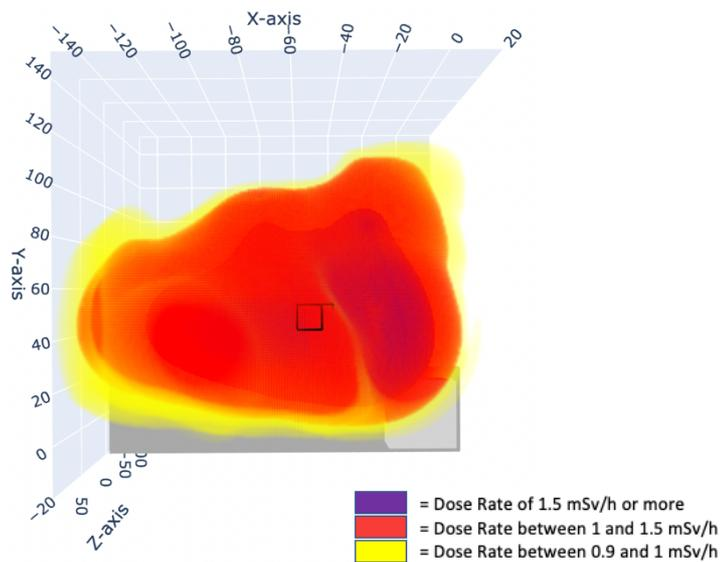
Figure 36: Interpolated visualisation of the data without a lead screen. 40° tilted orientation of the C-arm, Acquisition mode
