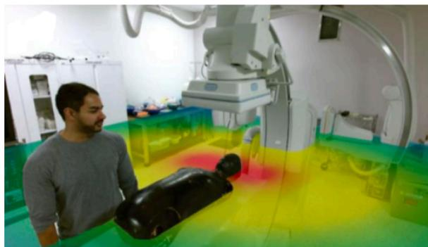
Figure 2: 3D (AR) scatter demo image featuring an anatomical phantom with a staff member in the image [34]
