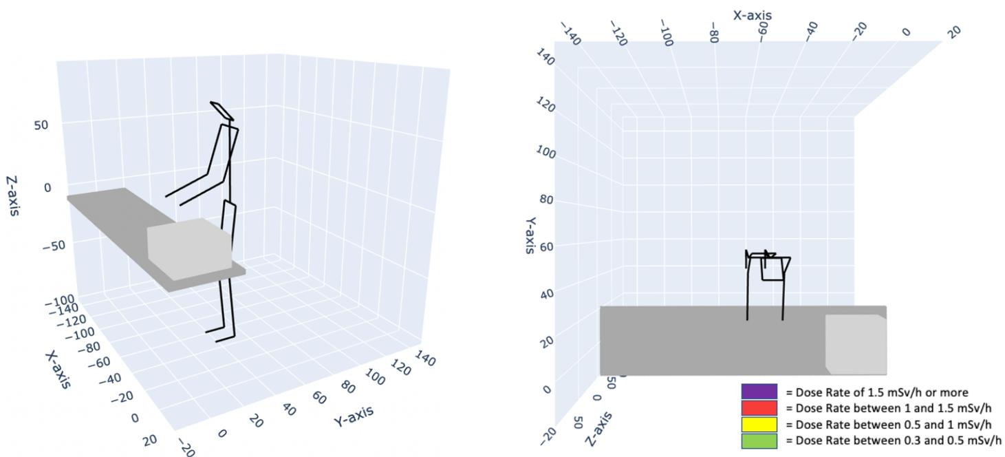
Figure 34: Interpolated visualisation of the data without a lead screen. AP orientation of the C-arm, Fluoroscopy mode
