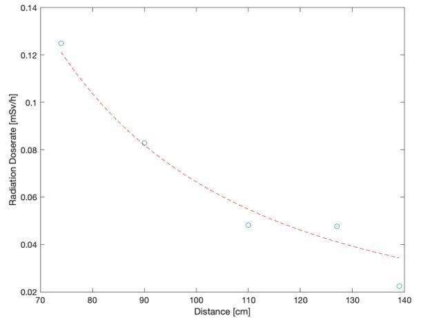
Figure 17: AP orientation C-arm, Fluoroscopy mode, No lead screen (measurements 105 cm above the ground)
