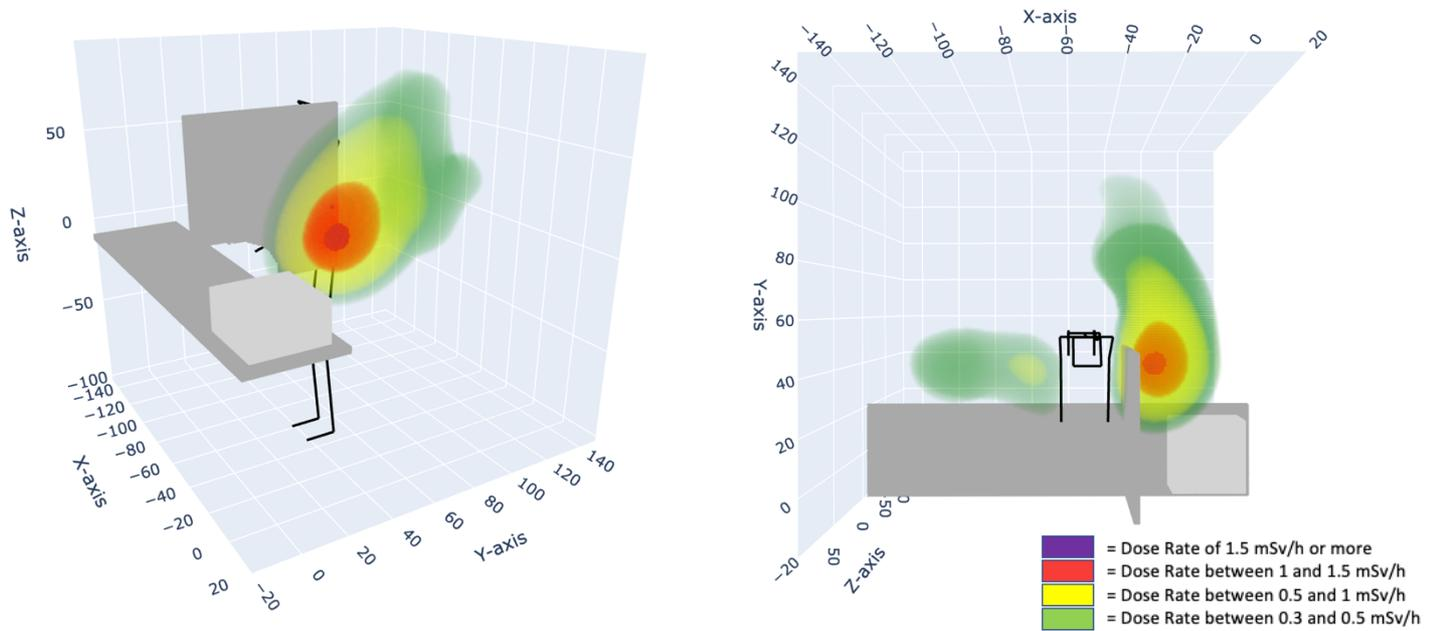
Figure 37: Interpolated visualisation of the data with a lead screen. AP orientation of the C-arm, Acquisition mode
