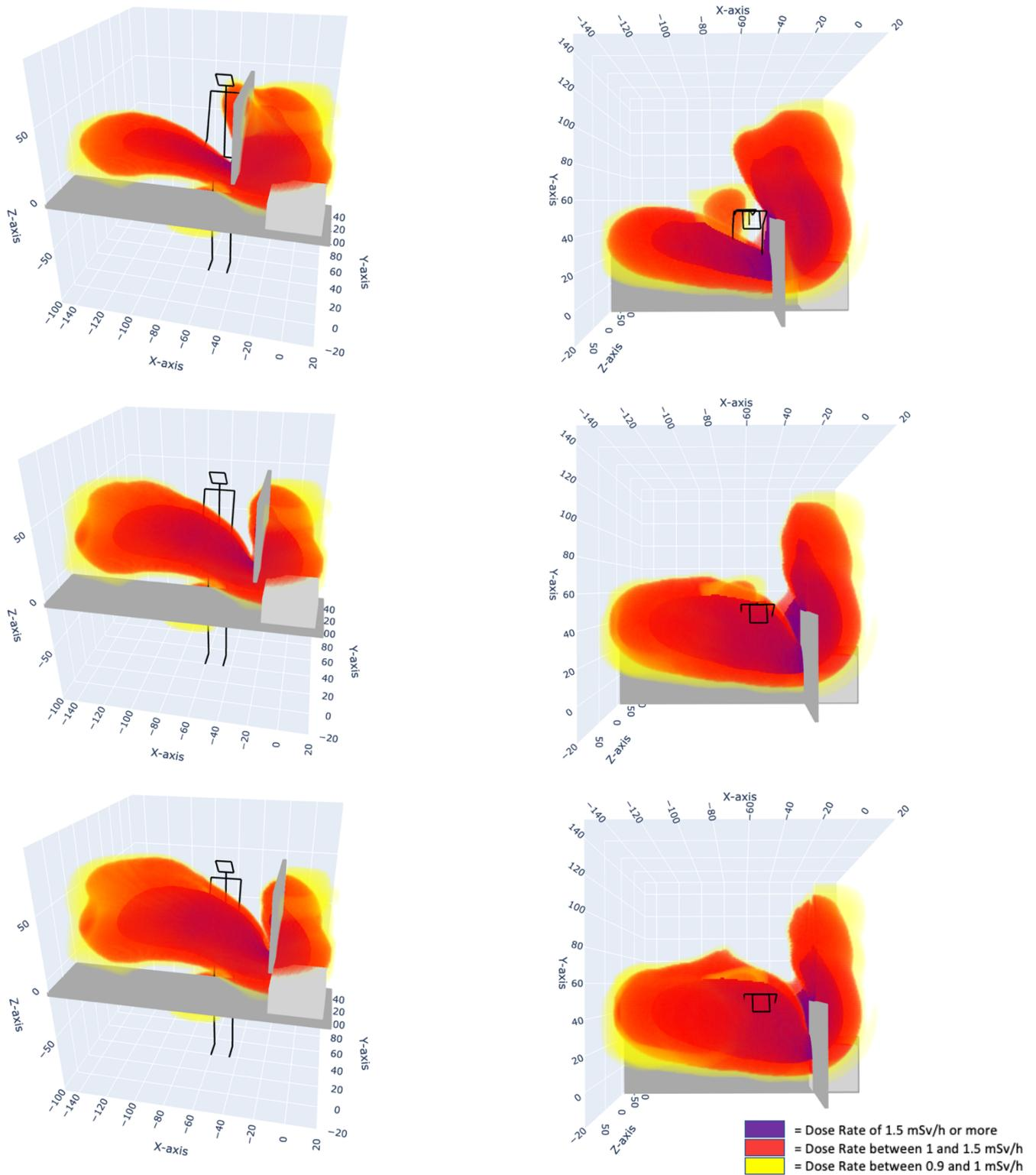
Figure 46: Estimated scatter patterns for three different lead screen positions with a 40° tilted orientation of the C-arm. Top: Lead screen positioned 20 cm from the edge of the phantom. Middle: Lead screen positioned 5 cm from the edge of the phantom. Bottom: Lead screen positioned 0 cm from the edge of the phantom.
