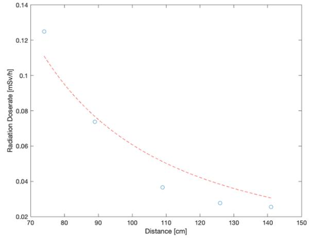
Figure 21: AP orientation C-arm, Fluoroscopy mode, With lead screen (measurements 105 cm above the ground)
