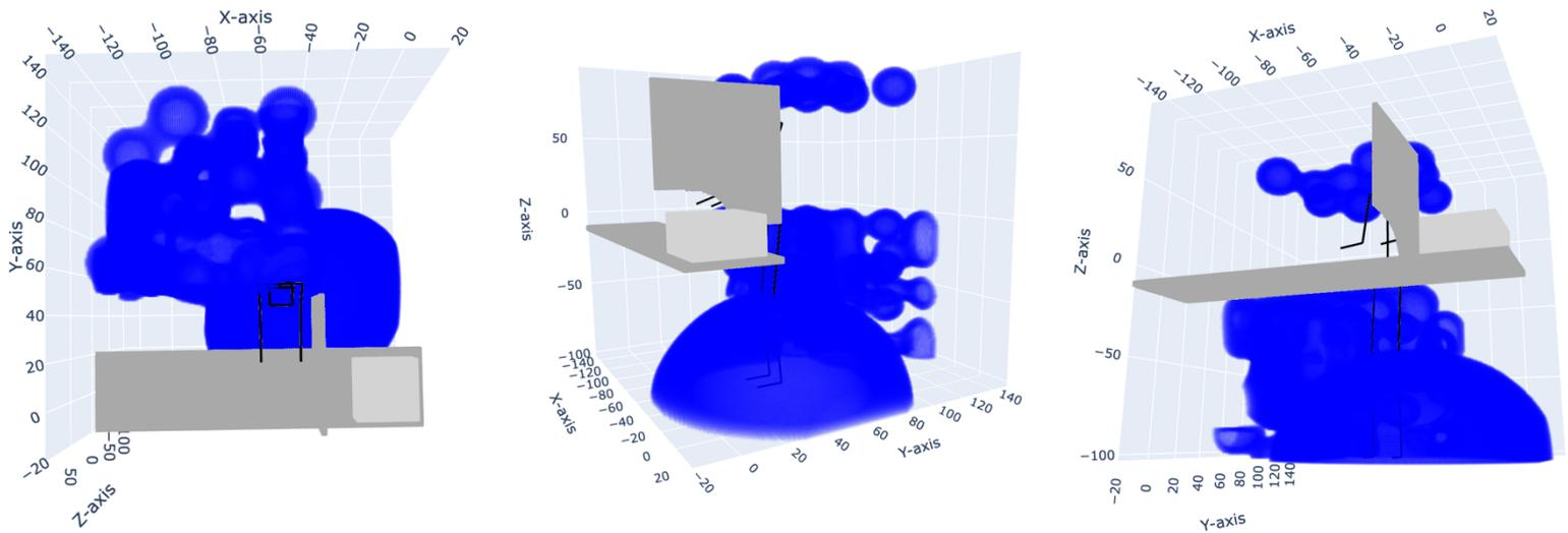
Figure 44: Interpolated visualisation of the inaccurately estimated values. 40° tilted orientation of C-arm, Fluoroscopy mode. Blue areas represent instances where the estimation provided a dose rate of at least 0.1 mSv/h lower compared to the measurements, indicating that the model overestimated the amount of radiation blocked. Conversely, red areas signify cases where the estimation yielded a dose rate of at least 0.1 mSv/h higher compared to the measurements.
