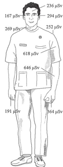
Figure 2: Graphic presentation of the mean values of doses per procedure found at the locations monitored for an interventional cardiologist [5]
