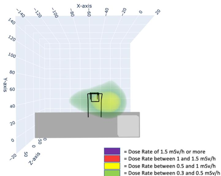
Figure 35: Interpolated visualisation of the data without a lead screen. 40° tilted orientation of the C-arm, Fluoroscopy mode
