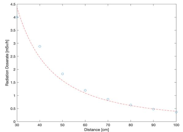
Figure 5: Plotted relation between the distance and the measured dose rate by the Raysafe
