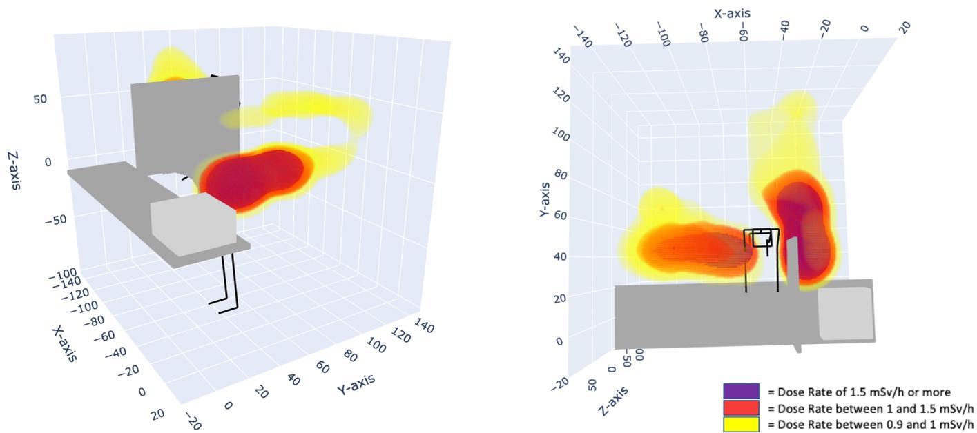
Figure 39: Interpolated visualisation of the data with a lead screen. 40° tilted orientation of the C-arm, Acquisition mode
