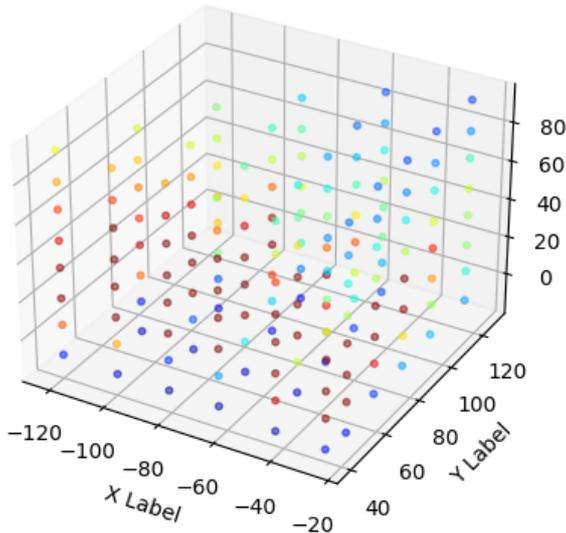
Figure 29: Measurement points; 40° tilted orientation, Acquisition mode, Without lead screen. The colour of the dots are dependent on the Doserate value, where dark blue is low and dark red is high.
