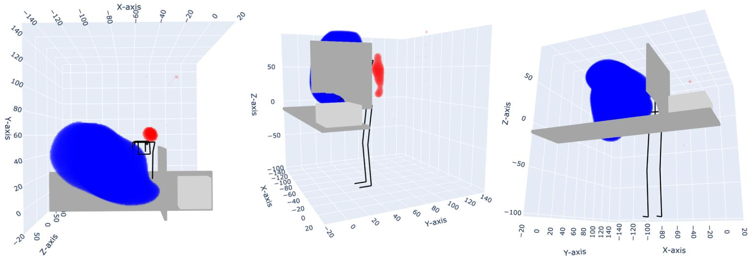
Figure 41: Interpolated visualisation of the inaccurately estimated values. AP orientation of C-arm, Acquisition mode. Blue areas represent instances where the estimation provided a dose rate of at least 0.1 mSv/h lower compared to the measurements, indicating that the model overestimated the amount of radiation blocked. Conversely, red areas signify cases where the estimation yielded a dose rate of at least 0.1 mSv/h higher compared to the measurements.
