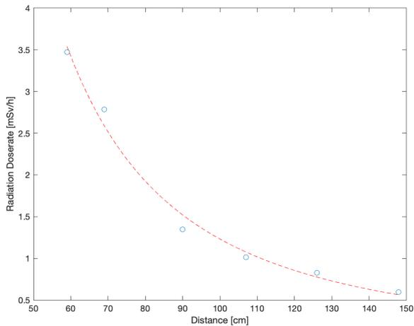
Figure 20: 40° tilted orientation C-arm, Acquisition mode, No lead screen (measurements 105 cm above the ground)
