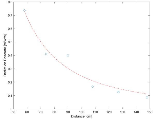
Figure 23: 40° tilted orientation C-arm, Fluoroscopy mode, With lead screen (measurements 105 cm above the ground)
