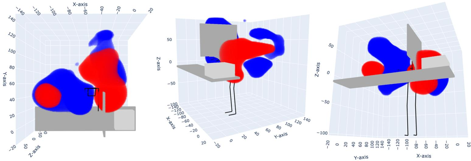
Figure 43: Interpolated visualisation of the inaccurately estimated values. 40° tilted orientation of C-arm, Acquisition mode. Blue areas represent instances where the estimation provided a dose rate of at least 0.1 mSv/h lower compared to the measurements, indicating that the model overestimated the amount of radiation blocked. Conversely, red areas signify cases where the estimation yielded a dose rate of at least 0.1 mSv/h higher compared to the measurements.
