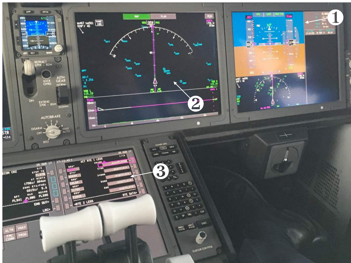
Figure E-3: Photographs from the Boeing 787 cockpit displaying the ❶ PFD, ❷ ND and a ❸ virtual CDU.
