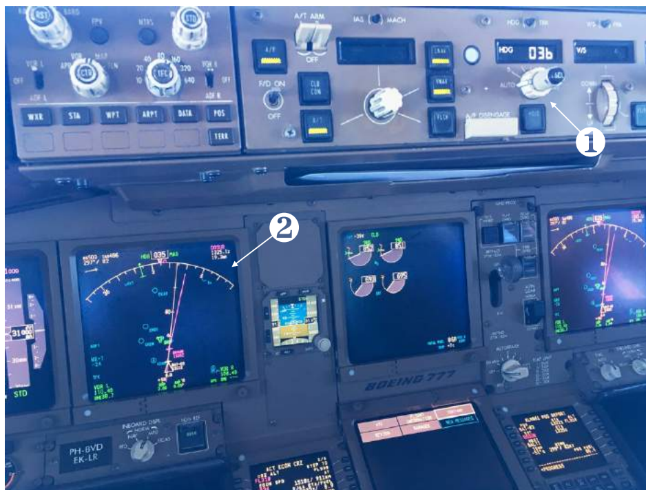
(a) ❶ (Rotary controller) commanding the heading select mode on the MCP. ❷ ND on the main instrument panel.
