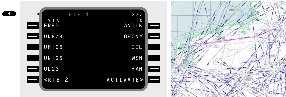
Figure 2-6: Example lateral flight plan definition on the ① RTE page for a route from Amsterdam to Hamburg, entirely based on airways and waypoints [25]. 2
