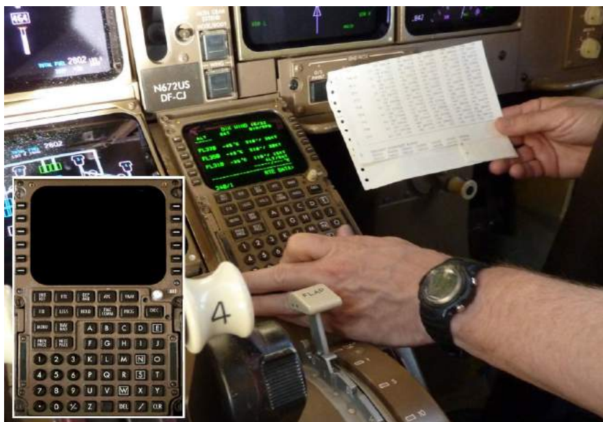
Figure 1-1: Pilot interacting with control display unit (CDU), entering en-route wind information (inset: Boeing-style CDU interface showing the conventional alphabetic keyboard and button interface) 1
