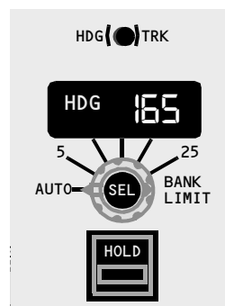
(a) Mode control panel (MCP) showing the heading select and hold interface [25]
