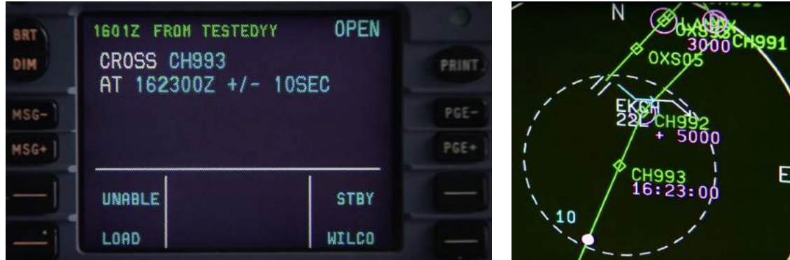
(a) Airbus A320 controller-pilot data link communications (CPDLC) display showing an incoming request to cross the CH993 waypoint at 16:23:00 with a tolerance of only 10 seconds. [2]
