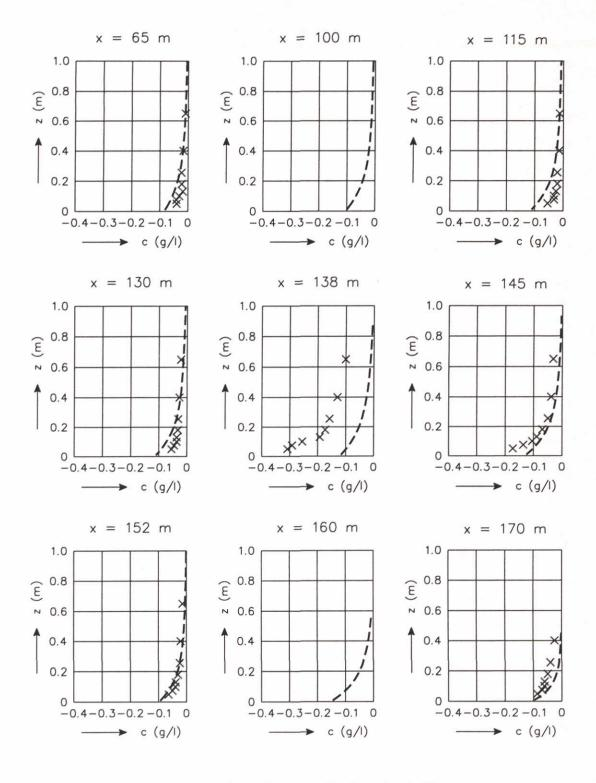
x measured sediment concentration test 1B--- computed sediment concentration
