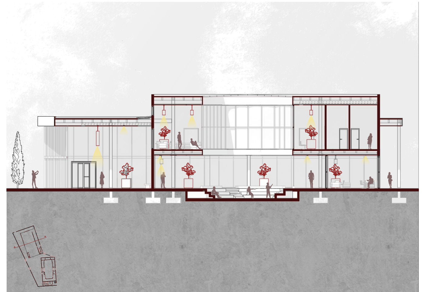
Figure 39. Lateral section of the public hall drawn in 1:200 scale
