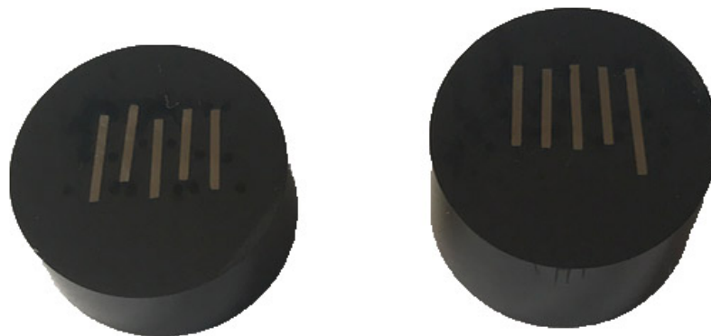
Figure E3: Substrates in epoxy mount
