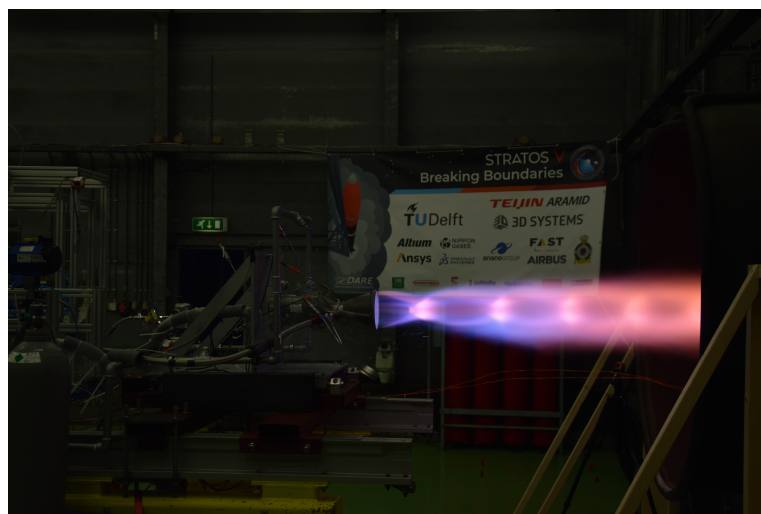
Figure 5.6: Hot-fire of the DLX150B "Firebolt" LOx/Ethanol engine developed by Delft Aerospace Rocket Engineering (Delft Aerospace Rocket Engineering, 2024)
