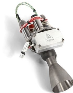
Figure 1.1: Dawn Aerospace B20 N_2O/C_3H_6 Thruster (Dawn Aerospace, 2025)
