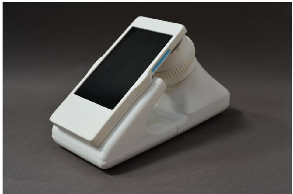
Fig 8. Motorized prototype with automated x-y movement of blood sample, which enables fast acquisition of large number of images.
