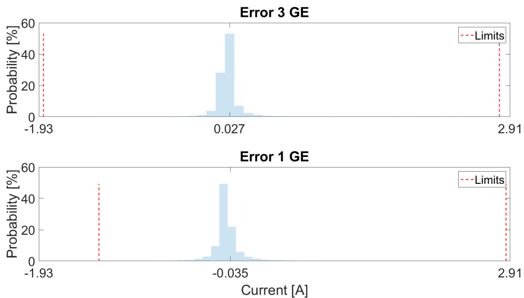
Figure 4.57: Histogram of current amplitude error distribution of both methods.
