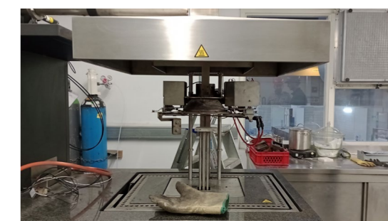
Figure 2.36: Cone Calorimeter test at Efectis (Own work)
