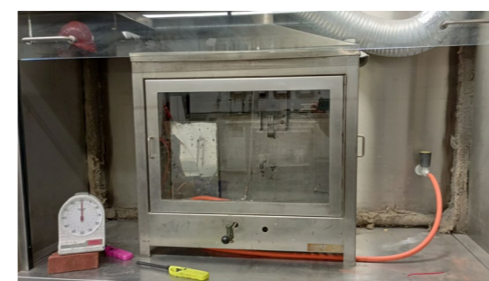
Figure 2.35: Ignitability test at Efectis (Own work)
