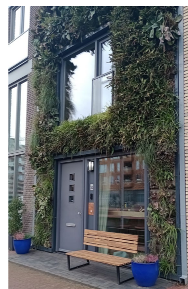
Figure 3.31: Row house. Sempergreen wall. Photos taken 23rd of January. Evergreens (Own work)
