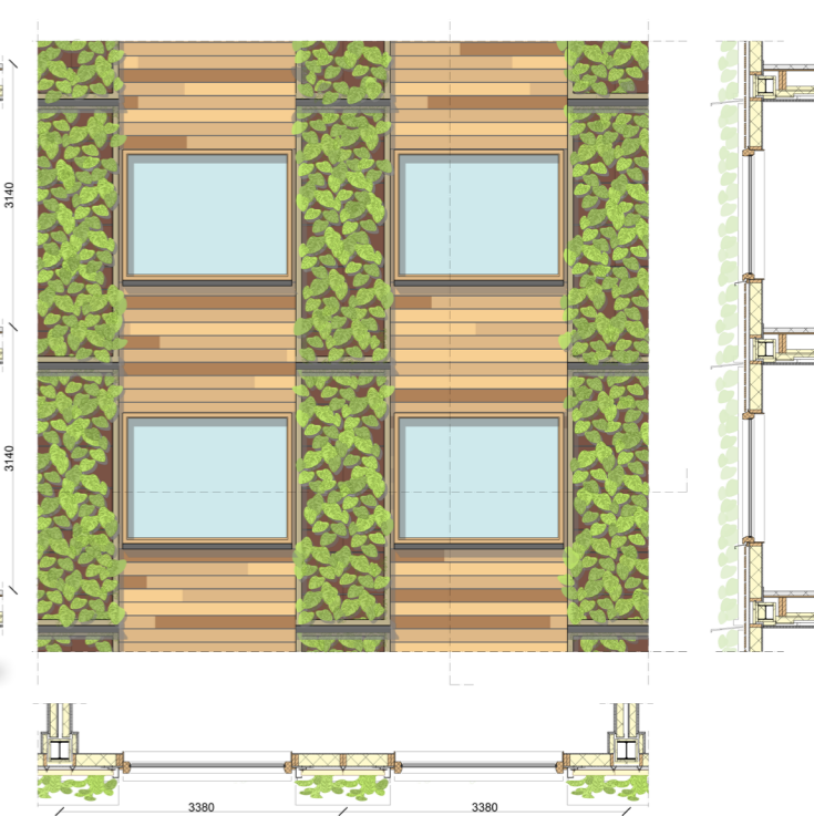
Figure 4.27: Lower risk façade view and sections with LWS 3. Drawn 1:20 scaled to 1:100 (Own work)
