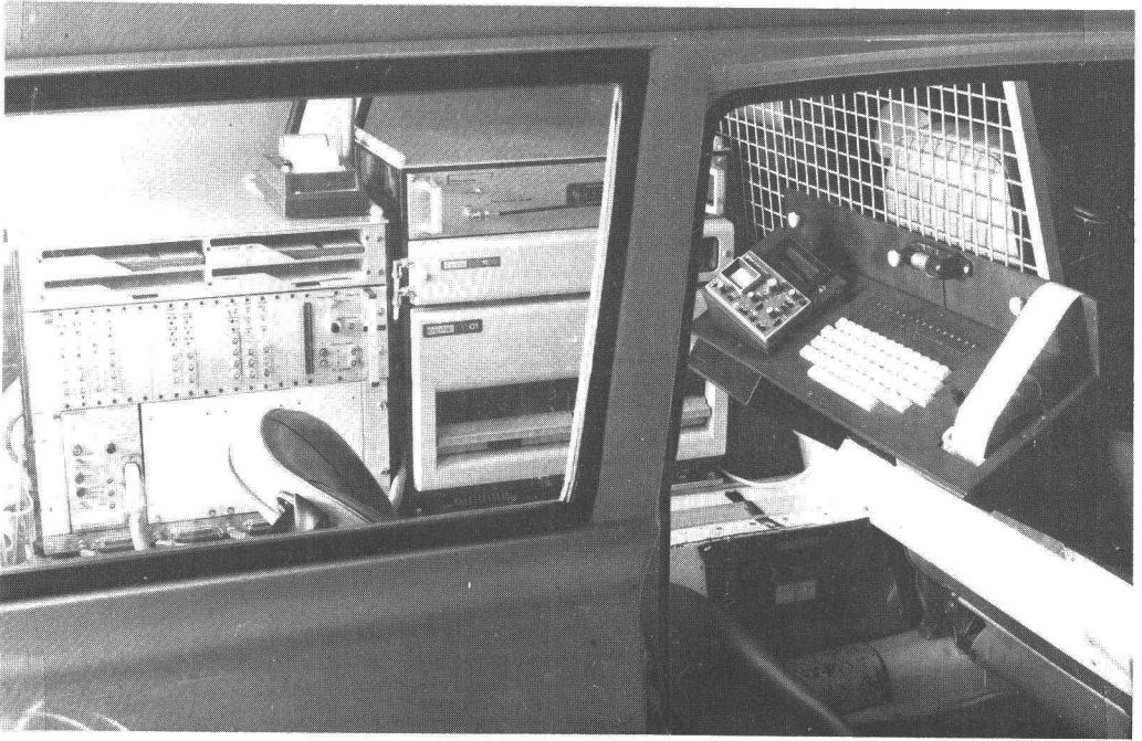
Fig. 4.4.1 The instrumented car with the on-board computer system. A minicomputer, floppy-disc unit and interface are placed directly behind the driver. A technician supervises the system with a keyboard, displays and a small printer. An experimenter uses a push-button unit to label special events during driving.
