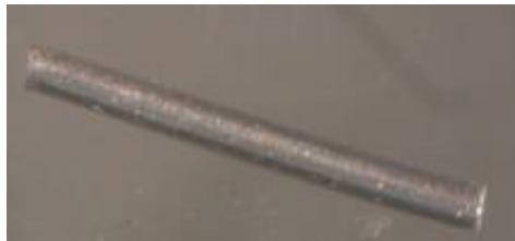
Figure 5-5: Aluminium wire particle of 10-mm length and 0.25-mm radius
