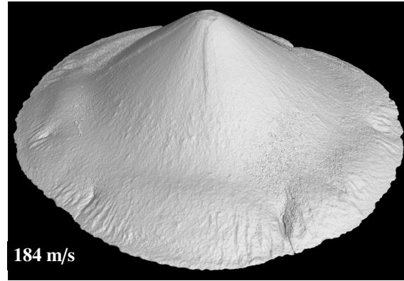
(a) An alumina ceramic cone, retrieved after a spherical impact experiment (E.P. Carton, TNO, personal communication, 2018). Figure was obtained by X-ray imaging (A. Thijssen, Delft University of Technology, personal communication, 2018).
