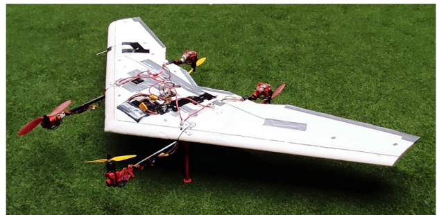
Fig. 1 A picture of the dual-axis tilting rotor quad-plane used as test bench for the CA methods
