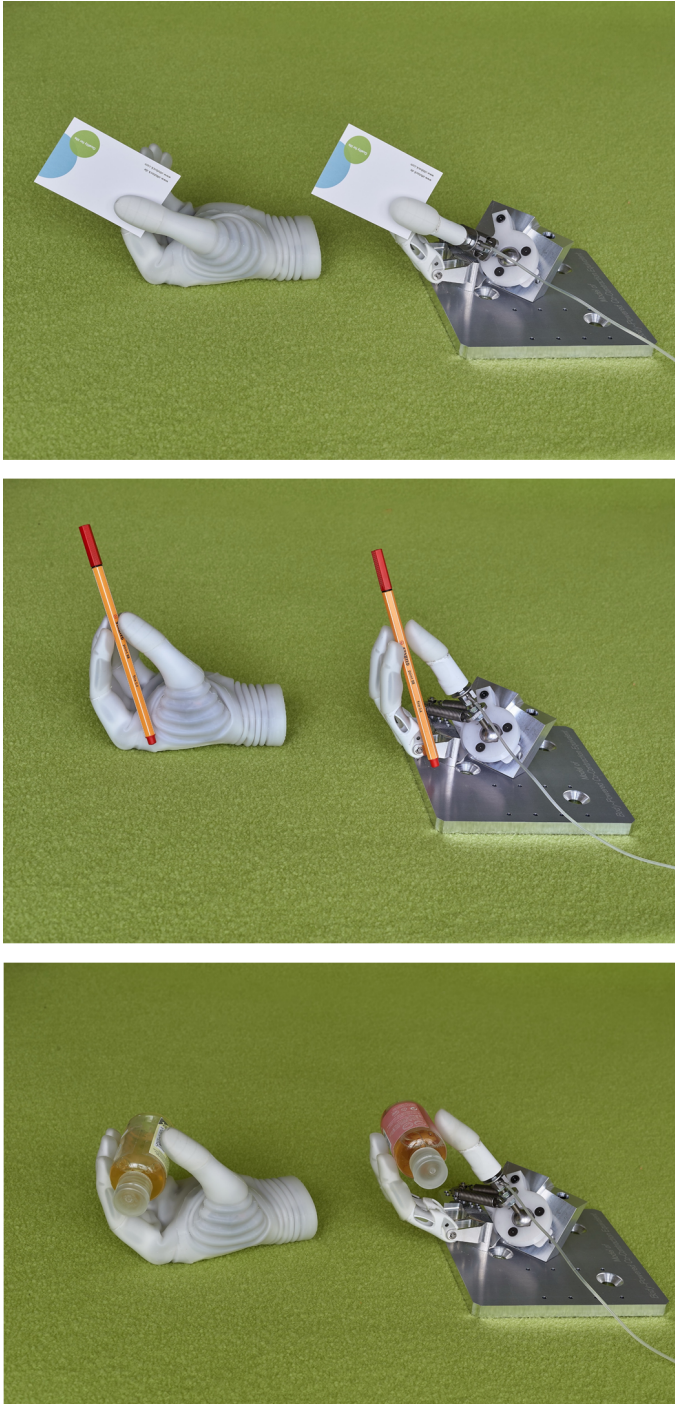
Fig. 8: Comparison of the developed device and the Michelangelo Hand by means of manufactured models in practice regarding the lateral pinch grip (top), the opposition pinch grip (middle) & the opposition power grip (bottom)
