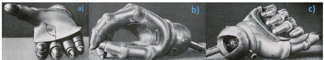
Figure 28: Hand of Troendle showing the finger alignment (top), a pinch grip (middle) and a power grip (bottom) (extracted from [51])
