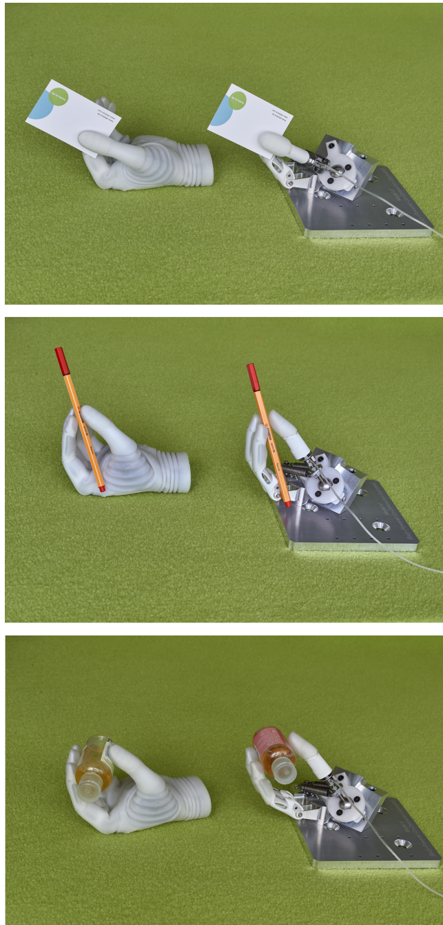
Figure 34: Comparison of the developed device and the Michelangelo Hand by means of manufactured models in practice regarding the lateral pinch grip (top), the opposition pinch grip (middle) & the opposition power grip (bottom)
