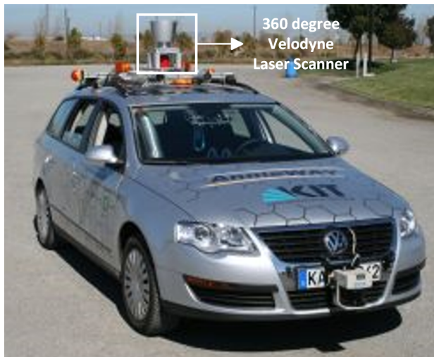
Fig. 1. The AnnieWAY Autonomous System Platform used by KITTI [18].
