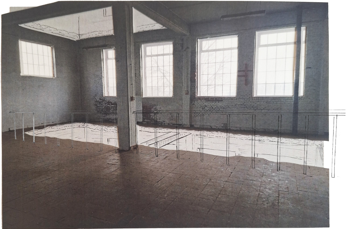
Figure 4.11 | Safety. Barrier in front of opened floor structure for increased porosity.
