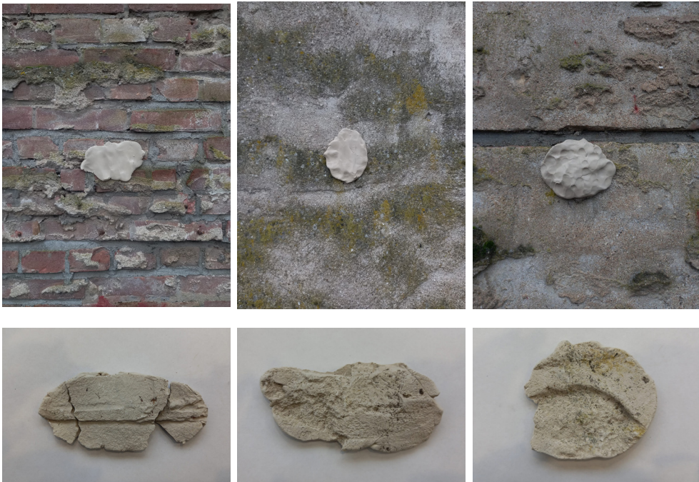
Figure 3.23 | Texture. Facade materials of Keileweg 26-29 have a rough texture, welcoming algae and lichen.
