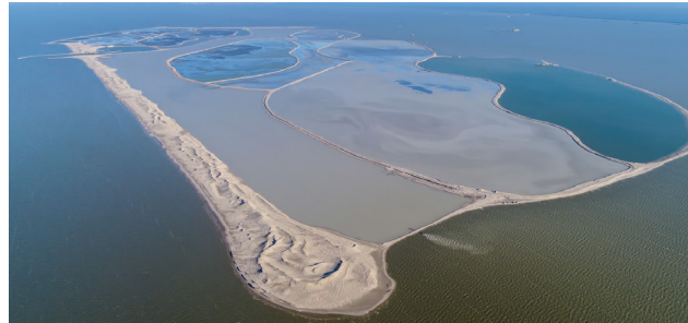
Figure 1.17 | Aerial photo after construction of the dams. The Marker Wadden were created by moving soil. (Natuurmonumenten, n.d.)
