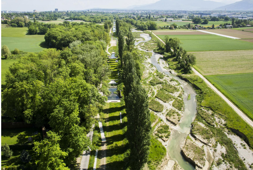
Figure 1.10 | River Aire. Two years after the construction of the grid the river had formed a new meandering. (Fabio Chironi, 2015)
