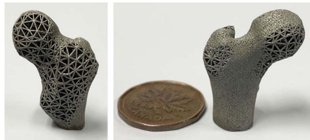
Fig. 16 A bone model with lattice structure generated by our approach as shown in Fig. 12—the metal model is fabricated by a SLM 3D printer
