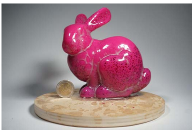
Fig. 15 A bunny model with lattice structure generated by our approach as shown in Fig. 12—the model is fabricated using a Connex Object350 3D printer
