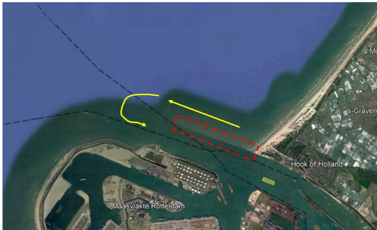
Figure 3.19 Trajectory of sediment movement in order to enters the Maasmond area. The Noorderpier structure (red dotted lines) prevent the sediment from move directly to the harbour area. After being discharged, the sediment is transported offshore until it passes the edge of the Noorderpier structure and return to the harbour area.
