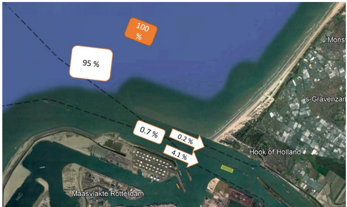
Figure 3.20 Return sediment percentage after being discharged at Verdiepte Loswal. Most of the sediments (95%) is spreaded at the North Sea while 0.7% of the discharged sediment deposits at the Maasmond. 4.1% of the sediment is transported back to the harbour area as sediment return while 0.2% of the sediment is transported to Nieuwe Waterweg.
