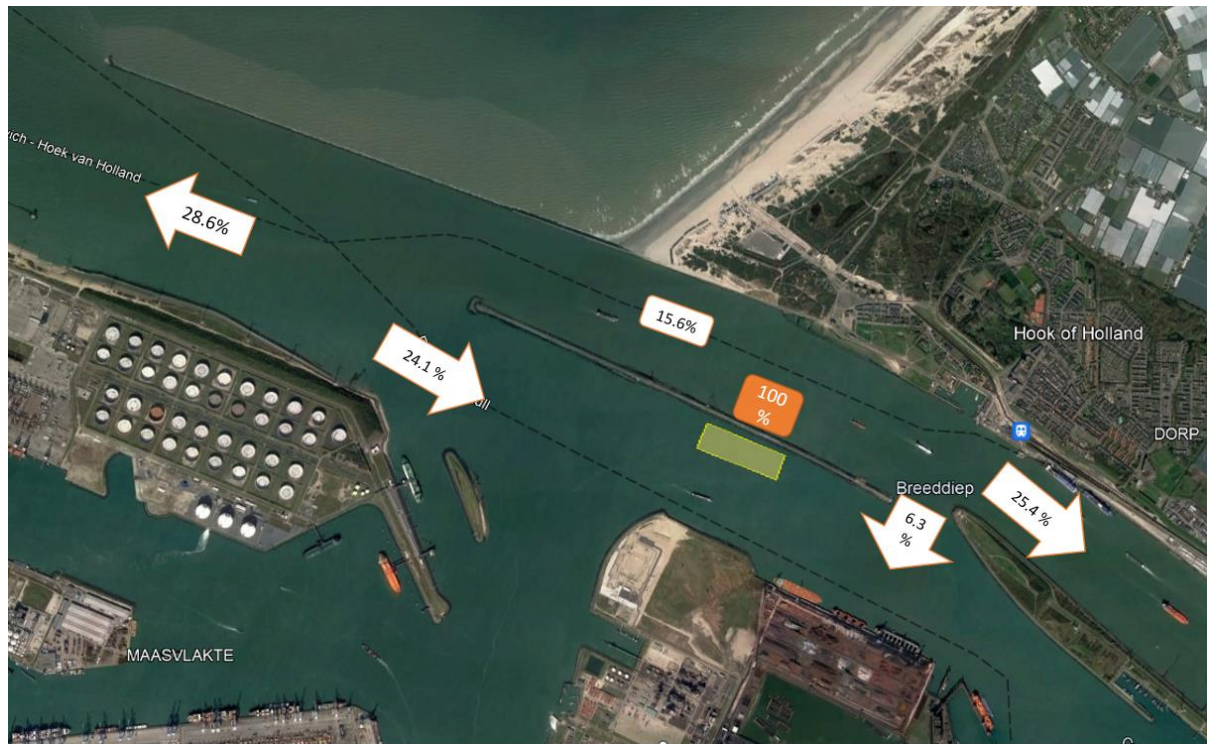
Figure 3.11 Percentage of sediment transported to each direction after discharged at Nieuwe Waterweg, considering continuous discharge over 24 hours. It is shown that 100% of the sediment is discharged at the discharge location (orange box) and then transported toward the directions represented by the white arrows. 15.6% of sediment is deposited at Nieuwe Waterweg (white box).
