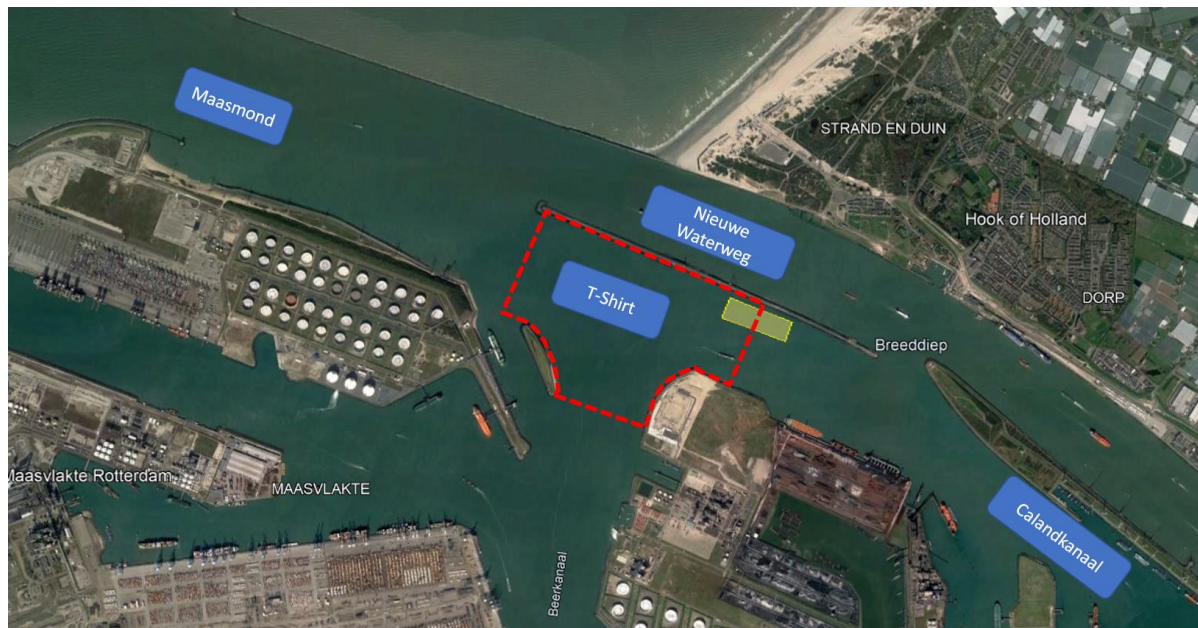
Figure 1.2 Study location (T-shirt) at the Port of Rotterdam is indicated by red dashed lines. Water injection dredging is regularly conducted in this area. Yellow coloured area shows the location of the sediment trap.
