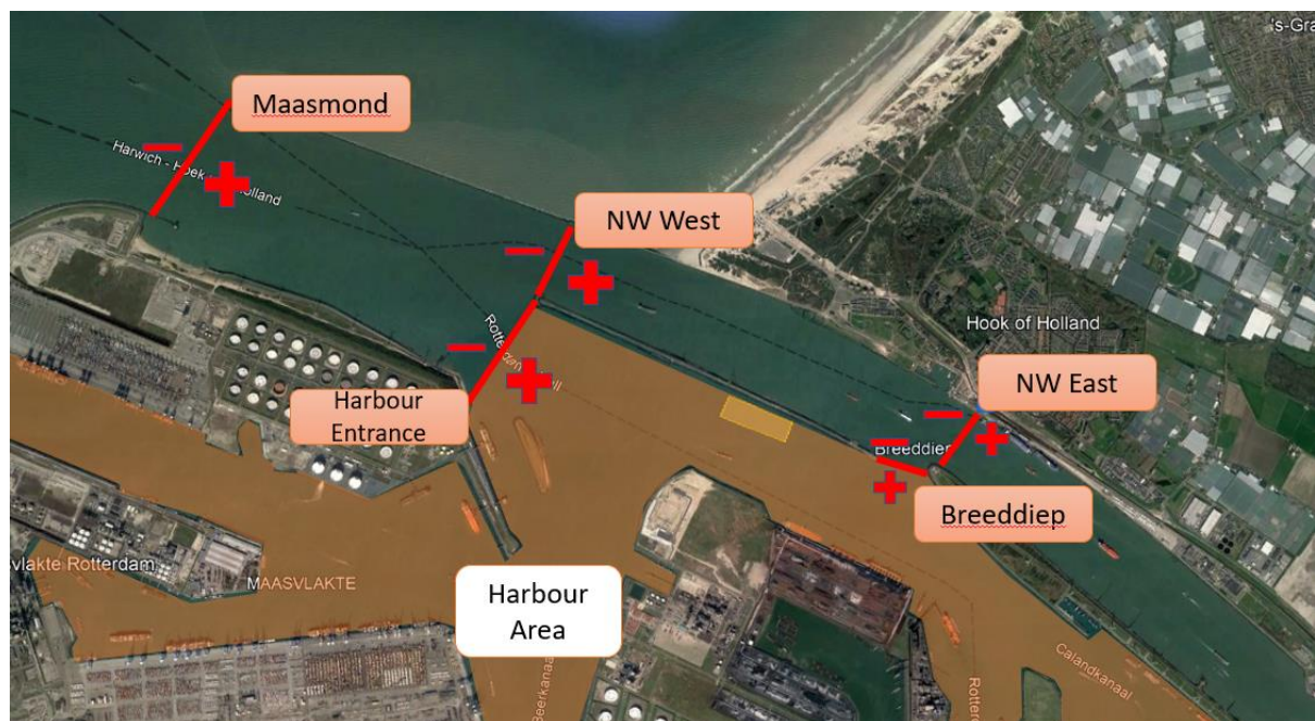
Figure 3.7 Locations of the Cross-sections. The positive and negative sign indicates the direction of sediment transport through cross-sections. Brown coloured area indicates the harbour area in this thesis, where sediments transporting back to this area is counted as a sediment return.
