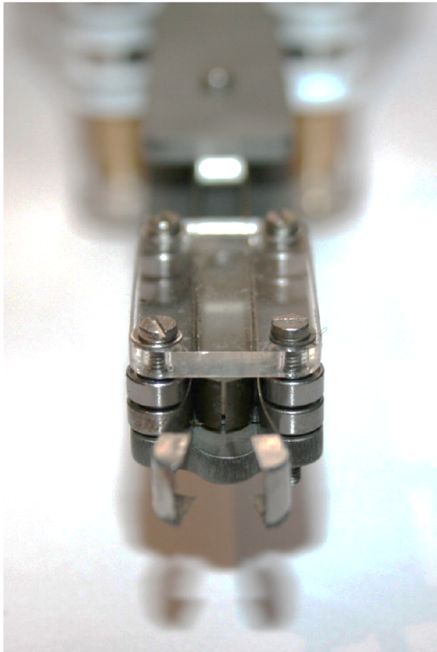
Figure 38 Front view of prototype tip; clearly visible is the gap between the scrapers.
