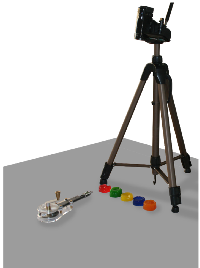
Figure 34 The experimental setup with the MultiBite prototype, camera and gelatine to test the working principle.
