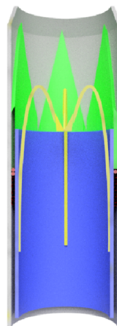
Figure 45 Cross-section of pre-concept 1, a conical cutter.
