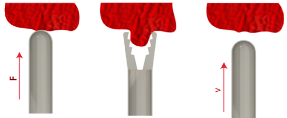
Figure 13 Solutions to tissue stabilizing, being: pressure, grasping, and shooting.
