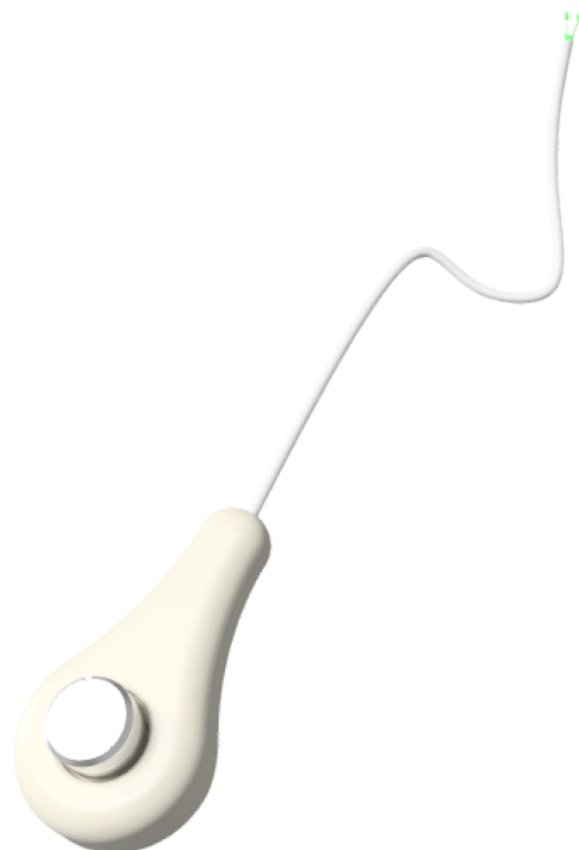
Figure 43 Visualization of a flexible 3 mm bioptome with handheld actuation.
