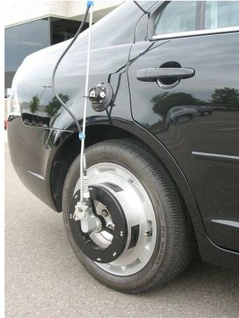
Figure 1.6: Measurement wheel able to measure the forces and moments in the rim.
