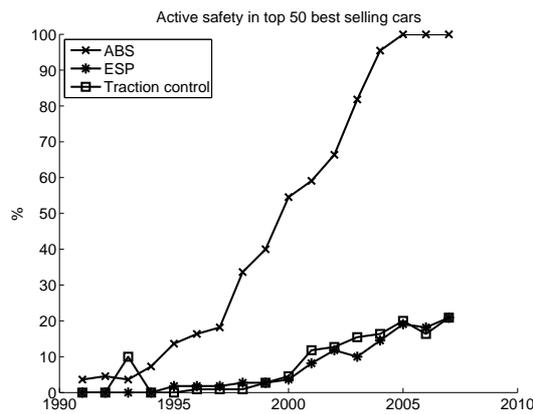
Figure 1.3: Percentage of the top 50 best selling cars fitted with electronic safety equipment. (Source [20])
