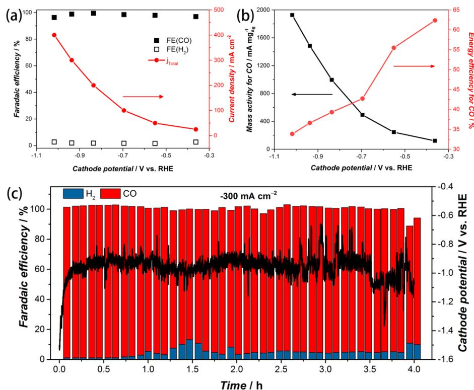
Figure 5. CO<sub>2</sub>ER performance of the Ag/MPL-3C electrode in a gas-fed zero gap flow electrolyzer. (a) Faradaic efficiency and total current density and (b) mass activity energy efficiency for CO. (c) Stability test at  $-300 \text{ mA cm}^{-2}$  for 4 h. The bar diagram represents the FE (left y-axis) of CO (red) and H<sub>2</sub> (blue), and the black line represents the cathode potential (right y-axis).
