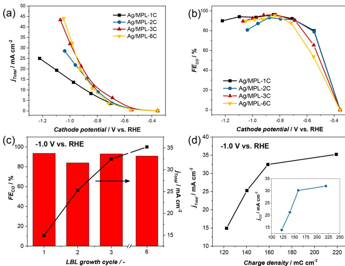
Figure 4. CO<sub>2</sub> electrochemical reduction performance of Ag/MPL-*n*C electrodes. (a) Total current density, (b) FE for CO, and (c) their LBL cycle dependency at -1.0 V vs RHE. (d) Variation of  $j_{\text{Total}}$  and  $j_{\text{CO}}$  with the electrochemical active surface area (EASA) at the same potential.
