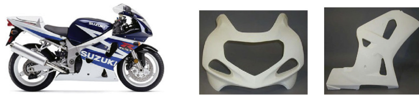
Fig. 8. Suzuki GSXR600 motorbike (left) and its front head cover (middle) and lower fairing (right) ([28], with permission).
