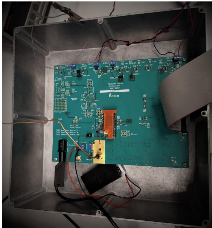
Figure 4-4: PCB inside the metal shield
