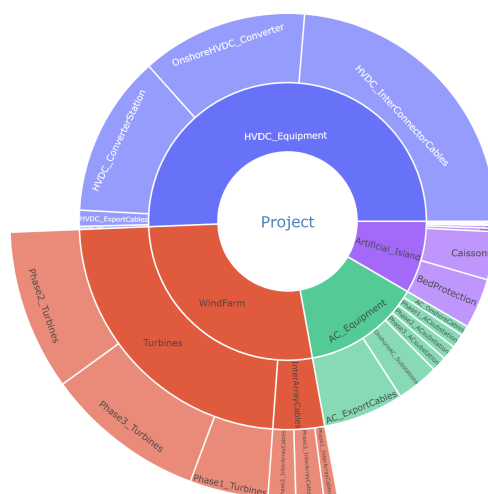
Figure C.10: Cost Distribution for PEZ Base Case with HVDC Interconnector
