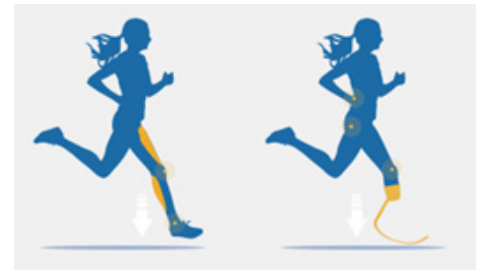
Figure 9: Energy storage in muscles versus in a prosthesis. Much like an able bodied runner's muscles, The prosthesis stores energy and absorbs impact that would have caused harsh reaction forces at various points on the amputee's body. (Ossur, 2021)
