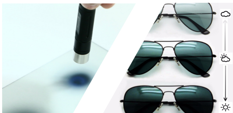
Figure 117. Sunglasses adjust transparency to UV intensity (AliExpress, n.d.)
