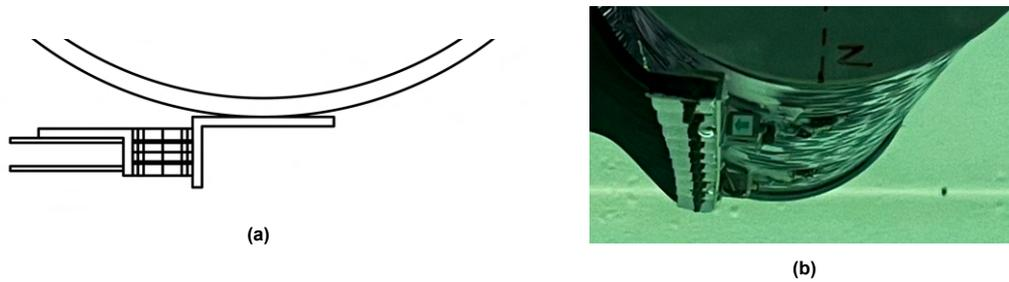
Figure 4.1: Technical drawing of the connection and the constructed connection in  $x, z$ -plane.
