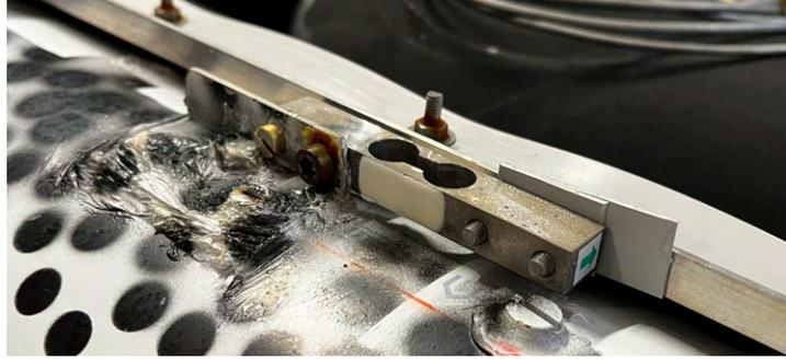
**Figure 5.8:** Force transducers are installed to have a positive sign for tensile loads and a negative sign for compression loads
