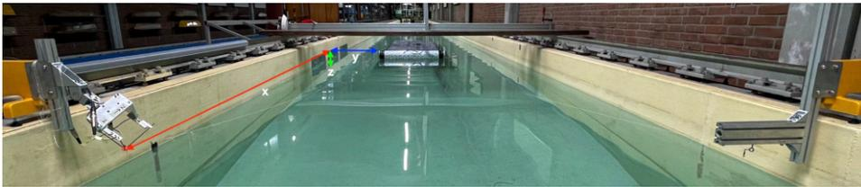
**Figure 5.4:** Visualization of the geometry of the mooring system in undisturbed water, front left and right mooring line are visible
