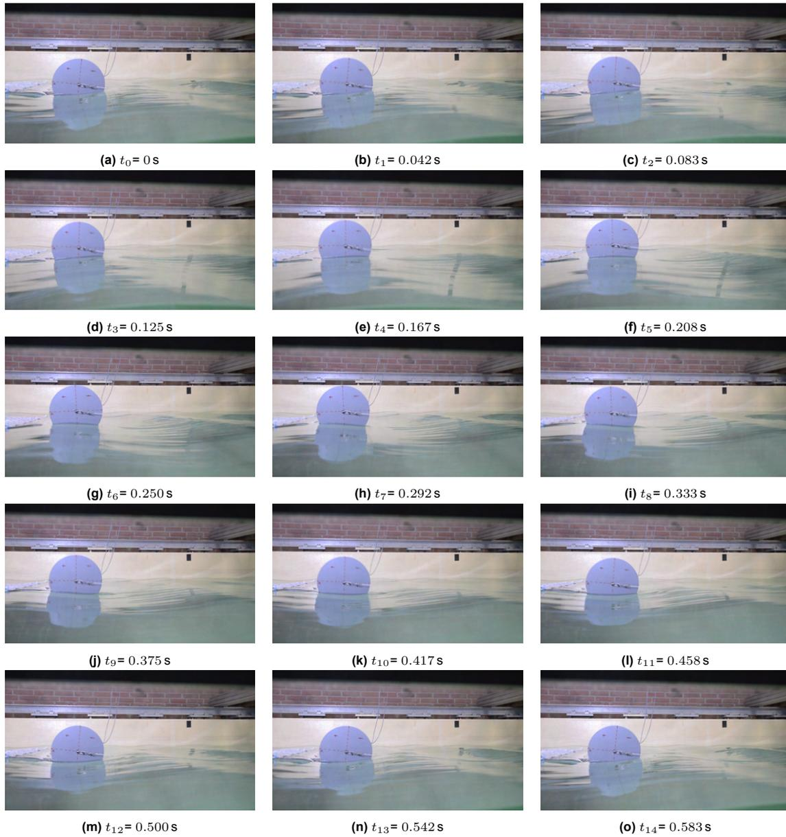
**Figure 6.15:** Visualization of wave and structure motion over one period excited by wave 4
