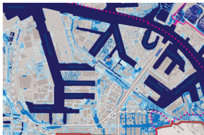
Scenario 2, flooding of the Lek at the 2050 safety level: Water level in the Noordzeekanaal under current conditions 0,8m - 1,3m NAP Return period: now, 1/10.000, in 2050 1/10.000
