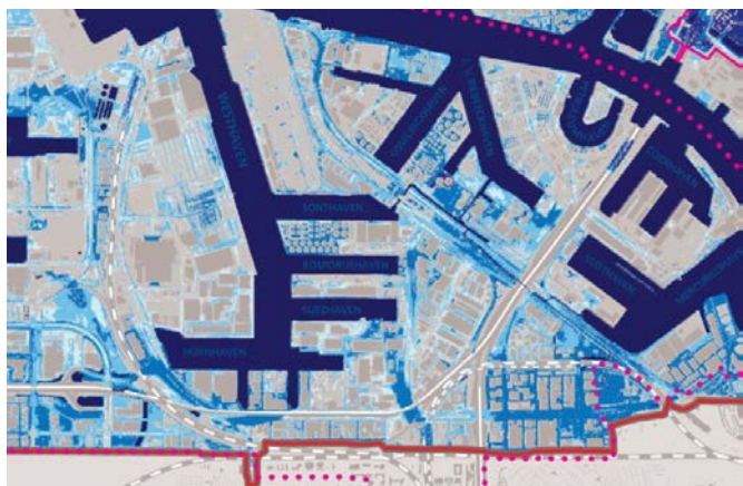
Scenario 3, breach at IJmuiden under the current safety level: Water level in the Noordzeekanaal under current conditions 0,9m - 1,4m NAP Return period: now, 1/10.000
