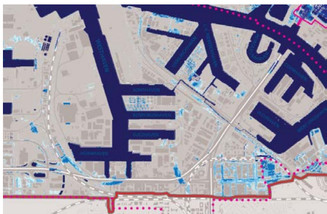
Scenario 1, flooding of the Lek at the current safety level: Water level in the Noordzeekanaal under current conditions at 0,4m - 0,9m NAP, Return period: now, 1/250
