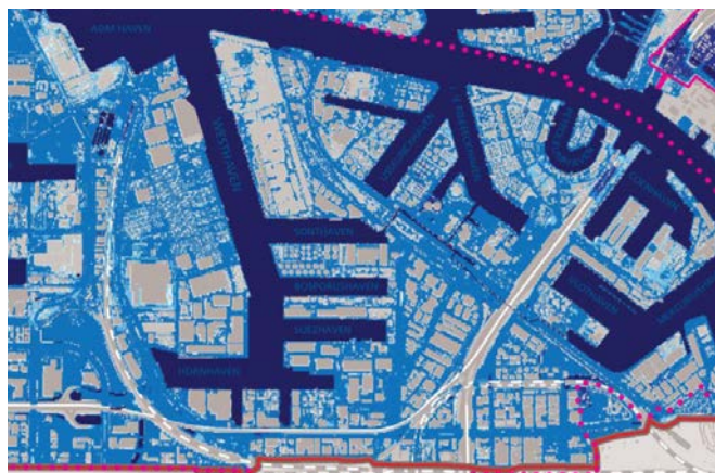
Scenario 4, breach at IJmuiden at the 2050 safety level: Water level in the Noordzeekanaal under current conditions: 1,5m - 2,0m NAP Return period: now, 1/100.000, in 2050 1/100.000
