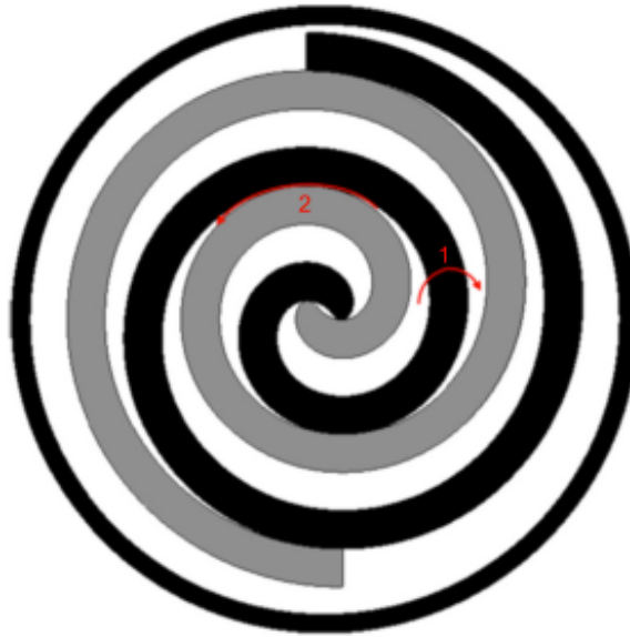
Figure B.2: Leakage path in a scroll expander. Lemort and Legros [27].
