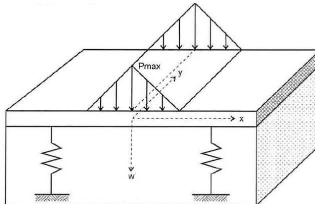
The maximum stress which occurs under the load can be calculated with:
