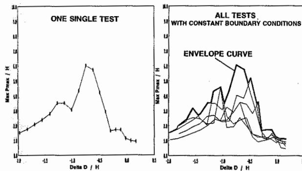
Fig. 4 Example for a local distribution of pressure data  $Max P_{max}/H$
