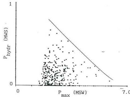
In the picture can be seen that the thicker the backwash layer the lower the maximum impact pressure.
