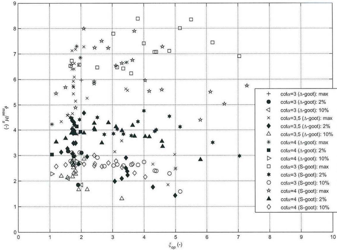
Klein Breteler in his analysis uses a Froude-Weber scaling to reduce the scatter which is caused by scale effects. Also the influence of the berm is taken into account which resulted in the following picture.
