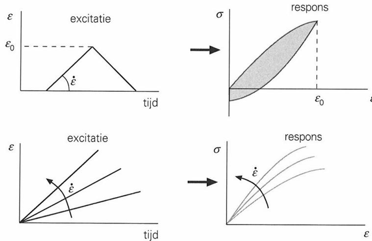
This means the value of the stress has a sine shape with the same frequency as the deformation but there is a phase difference  $\delta$ . The value of this  $\delta$  is always between 0 (elastic material) and  $\pi/2$  (liquid). Both  $\delta$  and  $E$  are dependent on the frequency, and for asphalt also on temperature. A part of the energy is dissipated.
