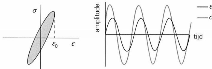
To better understand the behaviour of this material the stress response is rewritten (with  $\sin(a + b) = \cos(a) \sin(b) + \sin(a) \cos(b)$ ):
