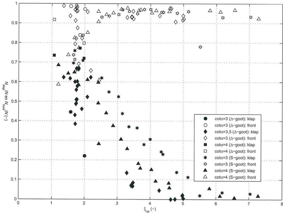
Where:  $\xi_{op} = \tan \alpha / \sqrt{s_{op}}$ ,  $\Delta$ -goot= Delta Flume, S-goot= Schelde Flume. The black dots represent a wave impact and the white dots a wave front.
