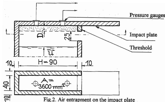
Fig.2. Air entrapment on the impact plate
