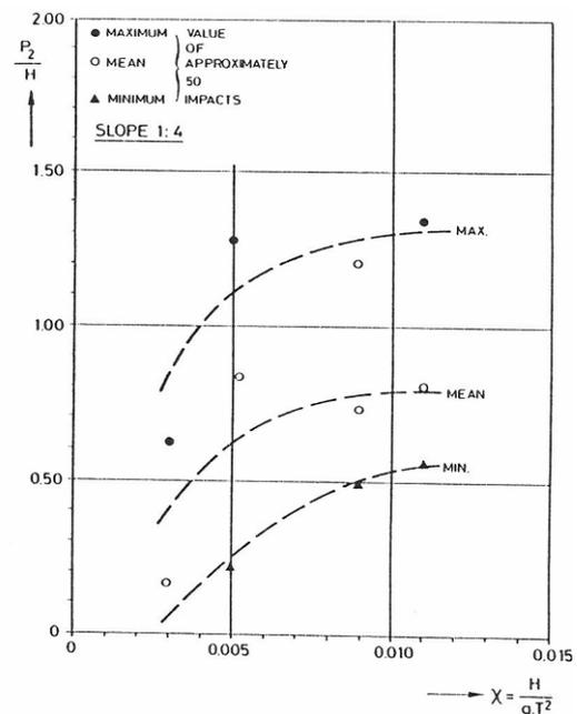
THE NORMALIZED "IMPACT" PRESSURE AT SLOPE 1:4, AS FUNCTION OF  $\chi$
