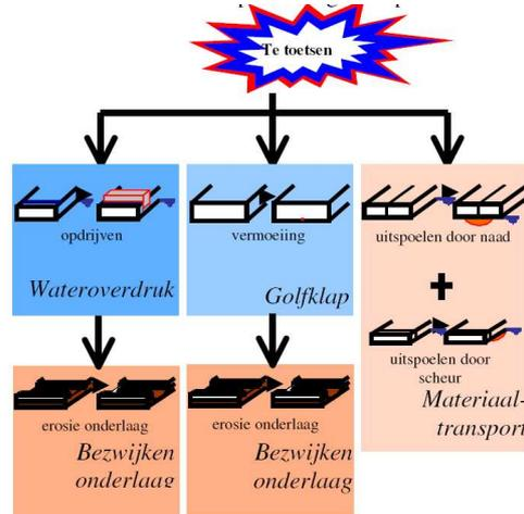
After failure for fatigue it is expected that cracks will appear in the layer and the layer will be ripped through because of that. When the layer is ripped through the revetment can slide down and/or sand will be washed out. This leads to exposure of the sub layer to erosion and thus the total collapse of the revetment.
