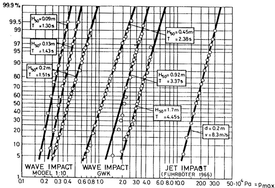
Comparison of results from water-jets, 1:10 scale test and full-scale tests
