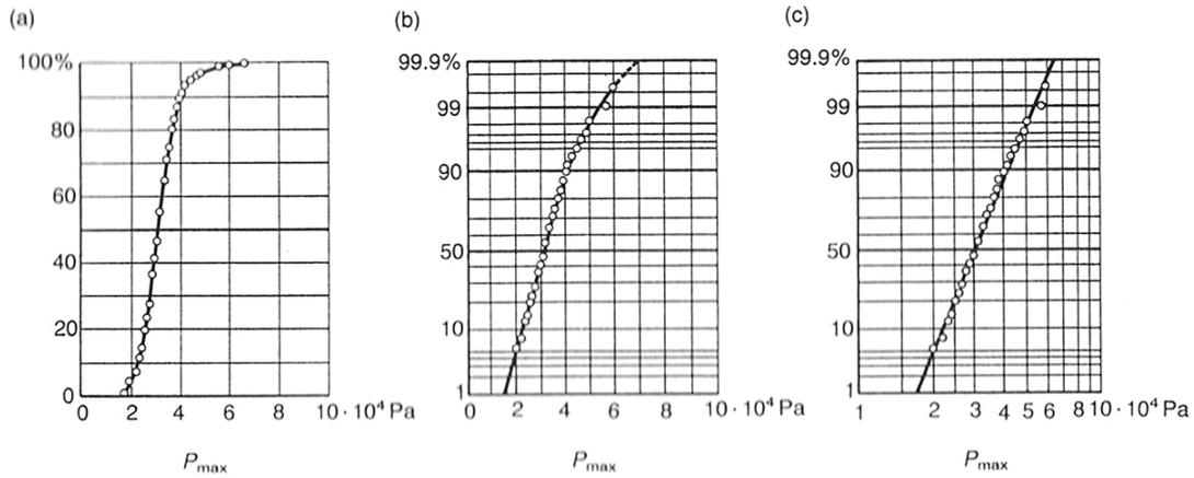
Probability distributions of impact pressures on smooth 1:4 slope (full-scale tests with regular waves  $H = 1.3$  m and  $T = 4.6$  s). (a) linear; (b) Gauss; (c) normal-log.
