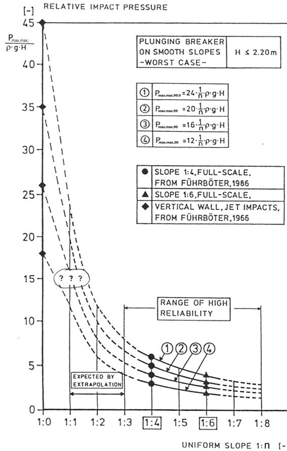
This graph shows the relation of the maximum impact pressure with the regular wave height. Sparboom (1991) based on Grüne (1988) made a comparison between wave height  $H_m$  (laboratory conditions) and  $H_s$  (real sea state conditions):
