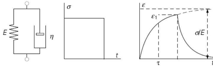
Both models do not fully describe the viscous-elastic behaviour. The first model fails to describe creep and the second model fails to describe the instantaneous deformation.
