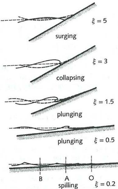
Plunging and collapsing breakers give the highest impact pressures, only the effects of these waves are treated in this report.
