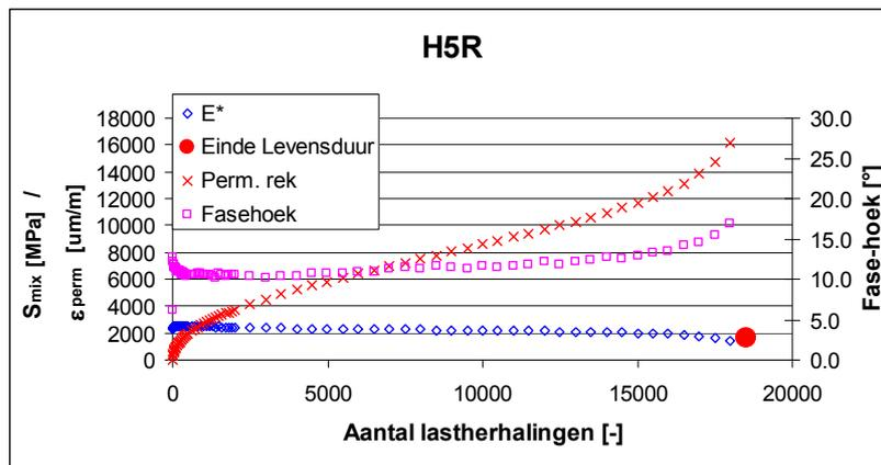
The fatigue properties are determined by testing several beams under difficult stress conditions. With the results of the tests a graph can be obtained.
