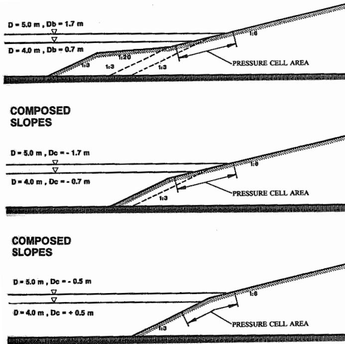
Fig. 1 Dyke cross-sections with berm and composed slopes, investigated in the LARGE WAVE CHANNEL (GWK)
