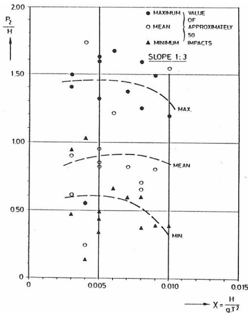
THE NORMALIZED "IMPACT" PRESSURE AT SLOPE 1:3, AS FUNCTION OF  $\chi$
