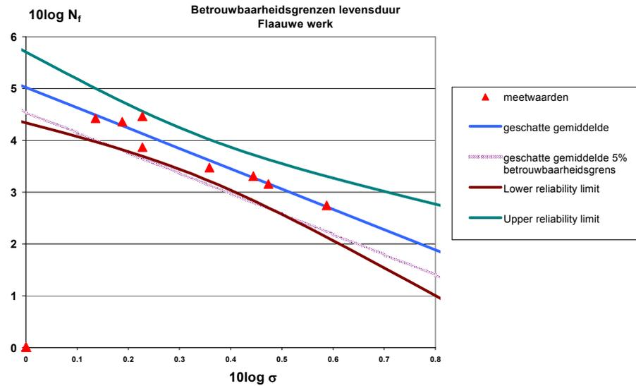
The graph shows the stress in relation with the number of load repetitions to failure. For all the weak spots these tests are done and put in the same graph. In this way a linear regression line of the fatigue property is obtained.
