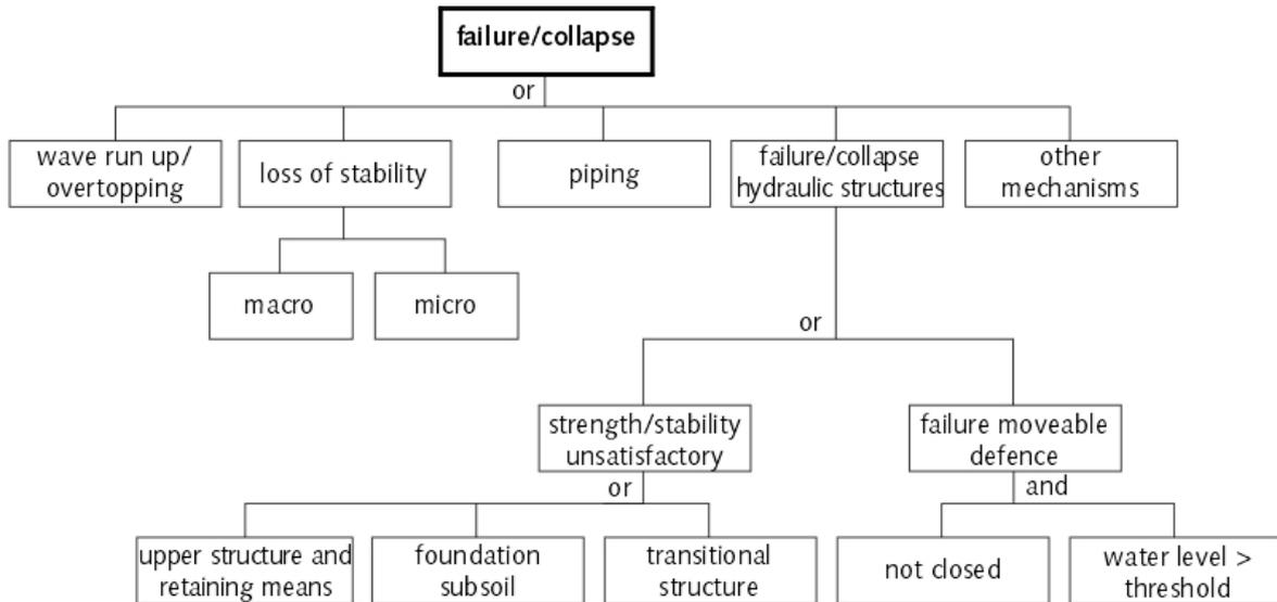
By assigning a probability of failure to each of the components of the fault tree insight is gained about the probability of failure of the top event. Also the weak spots in the construction become clear in this way of approach. The values of these loads are processed in the hydraulic boundary conditions mentioned earlier.
