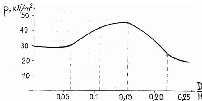
Fig. 4. Effect of dimensionless thickness ( $D/H$ ) on magnitude of impact pressure
