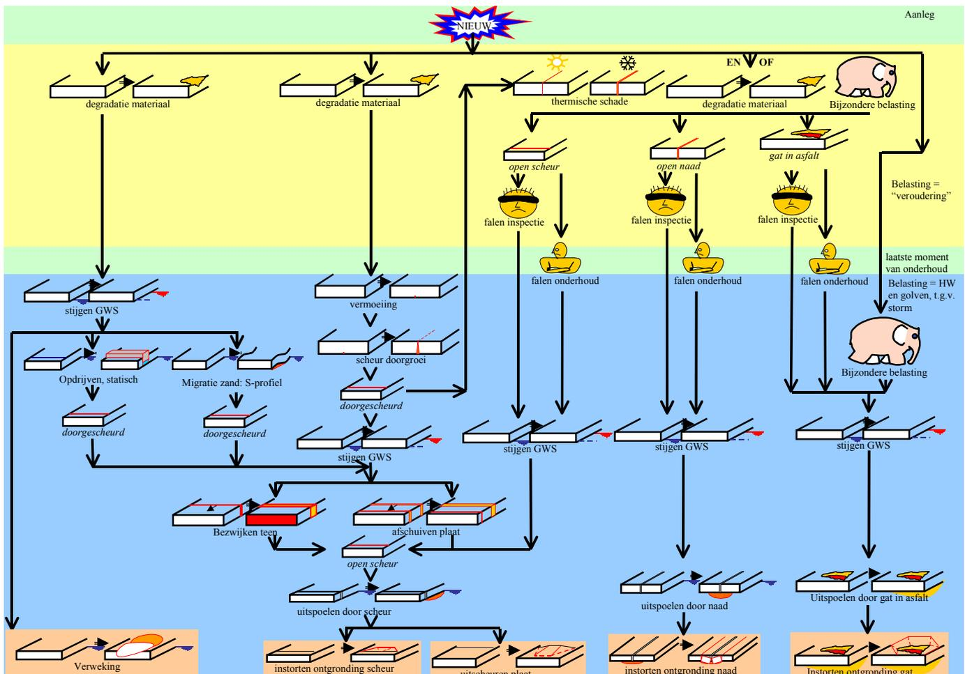
The revetment fails when 1 m<sup>2</sup> of the sub layer in the wave attack zone is exposed to erosion; at the bottom of the fault tree this is shown. The consequences of special loads are not taken into account.
