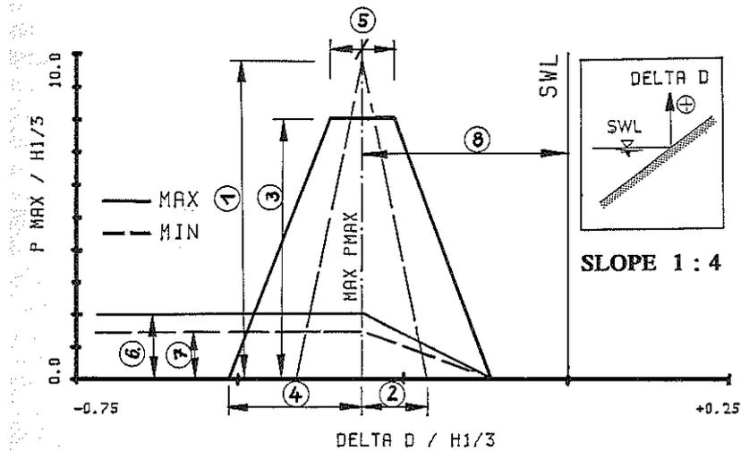
Fig. 17 "Dynamic" loading model for slope 1 : 4
