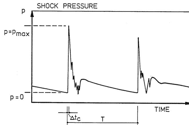
The maximum impact pressure is also dependent on the slope. This is explained by the influence of the backwash layer. Van Vledder concluded:
