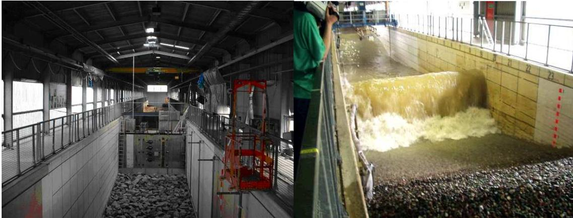
In 1983 Stive analyzed two series of full-scale measurements of regular waves breaking on a dike slope in the Delta Flume. The first series concerns a 1:3 slope of open stone asphalt revetment and the second concerns a 1:4 slope of a regularly placed artificial stone revetment.
