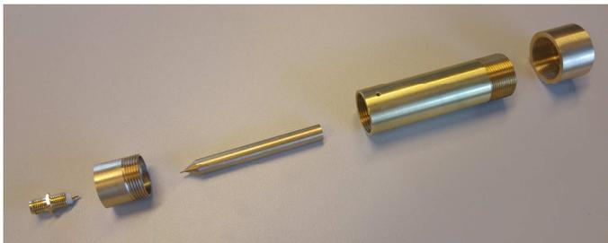
Fig. 1. Structure of the impedance probe.
