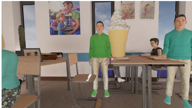
Figure 5: The setup for the environmental sound awareness test. The sound was presented from 90 degrees azimuth animal stimuli. Participants could achieve a visual reward when looking in the right direction.
