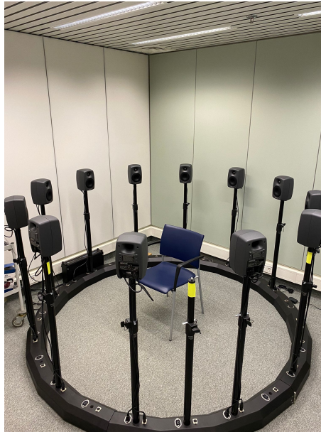
Figure 2: 12-array loudspeaker setup with 30 degrees distance in between.
