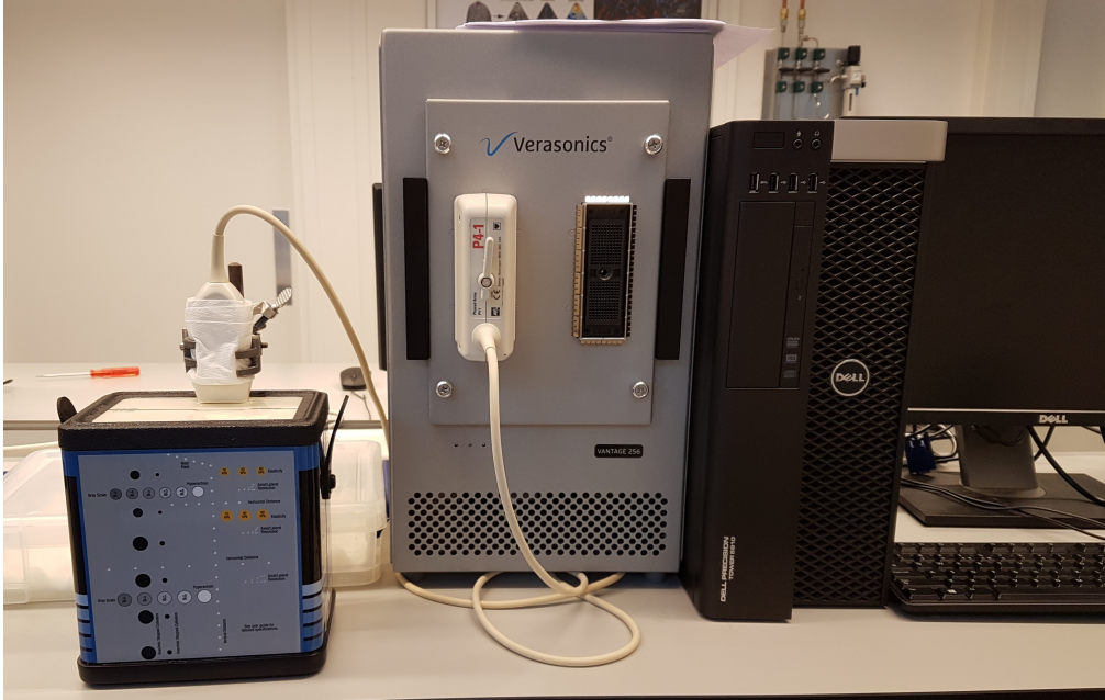
Figure 3.2: Experimental set-up. On the left the CIRS phantom can be seen with on top of it the P4-1 transducer. In the middle is the Verasonics and on the right the PC to which it is connected.
