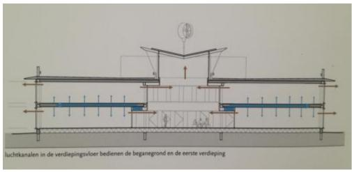
Figure 6.7: The ventilation system in the town hall according to the design
