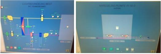
Figure 6.10: Control Maintenance and Operation System (Monitoring the Ventialtion)
