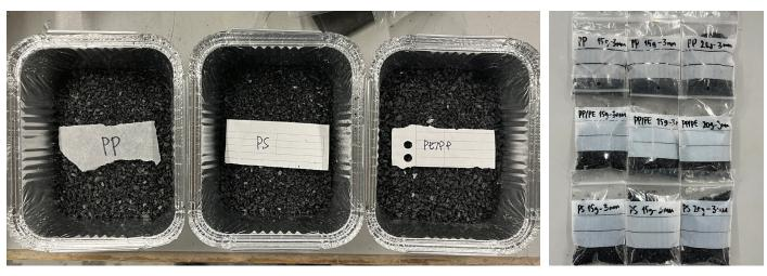
Figure 85: (1) Shredded 3 mm polymer batches for the PP, PS, PP/PE blend (2) 15-20 g injection-ready batches (Source: Author)
