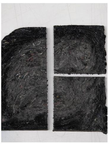
Figure 63: 50x50 mm transverse and longitudinal cut scenario of samples after processing (Source: Author)
