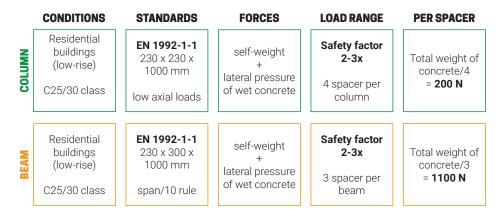
Table 24: Compressive strength simulation setup for column-beam applications (Source: Author)
