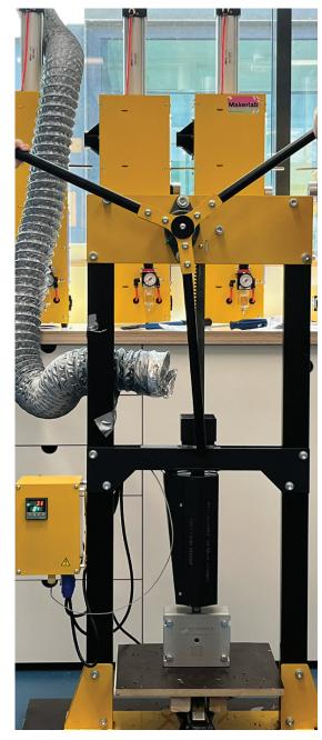
Figure 59: The Arbour Press Injection Machine injection molding setup (Source: Author)
