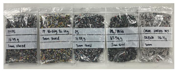
Figure 57: 3mm shredded polymer batches for processing (Source: Author)
