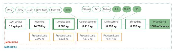
Figure 100: Recycling/Recovery rate for Module D1 (Thesis' scenario) and Module D2 (Industry scenario) (Source: Author)
