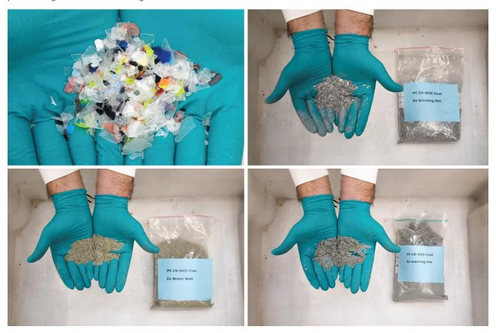
Figure 39: The reject fractions from various sorting steps of MEWA recycling facilities (Source: Author)
