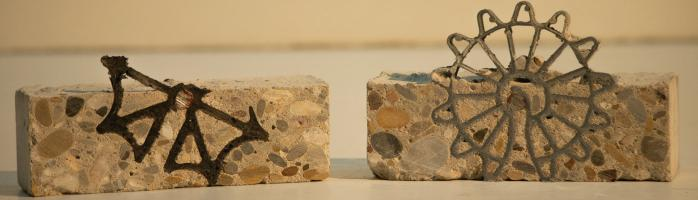
Figure 97: The penetration results on the cut-mockups of (1) fine (2) recycled coarse (3) regular coarse aggregates (Source: Author)
