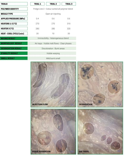
Table 11: First experiment setup with pneumatic plunger-type injection molding and parameter analysis (Source: Author)
