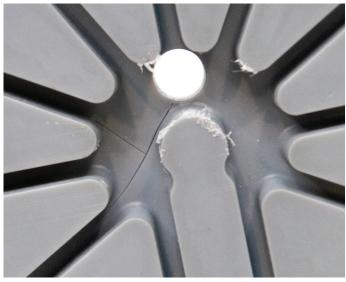
Figure 75: The crack formations on the upper plate resin mould (see right) and bottom plate resin mould (see left) (Source: Author)
