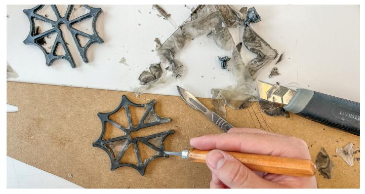
Figure 90: The setup for the removal of flashing for the succesful injection molded samples (Source: Author)
