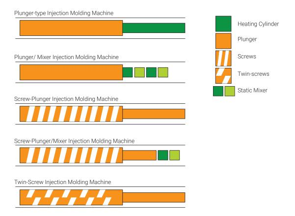
Figure 19: Schematic of different types of injection molding machines (Adapted from: Han et al., 1977)
