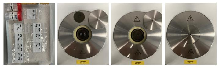
Figure 44: DSC preparation (1) selection of sample, (2) placing sample and reference pan, (3) closing the insulation lid, (4) closing the main lid (Source: Author)
