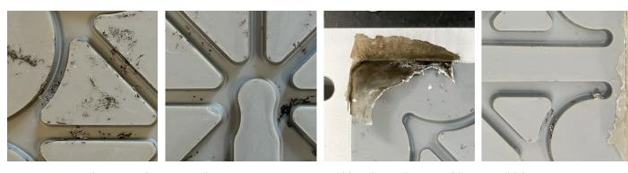
Figure 80: The deformation of the mould after 30 injection molding trials (1) surface deformation (2) cracking (3) flashing in-between two moulds (4) warping of the mould (Source: Author)
