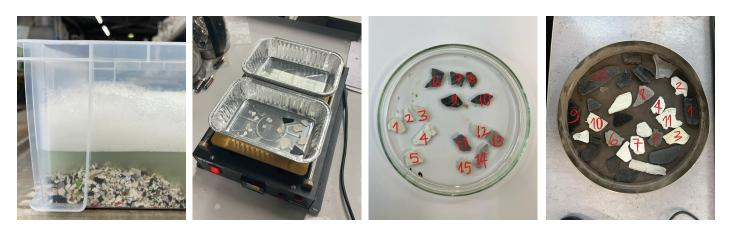
Appendix.10 FT-IR analysis preparation (1) washing samples with detergent, (2) drying the samples, (3)(4) numbering the sample before characterization
