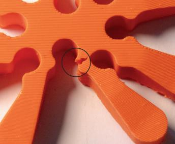
Figure 71: (1)The rebar retention mechanism tests and (2) Failed rebar test on the Spacer 8 (Source: Author)
