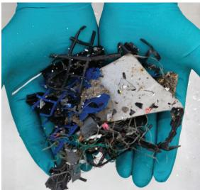
Figure 38: The reject fraction of Van Werven recycling facilities (Source: Author)
