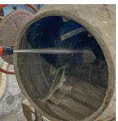
Figure 93: Material preparation steps (1) Collecting dry mass (2) Mixing dry materials (3) Adding water (4) Cleaning after use (Source: Author)
