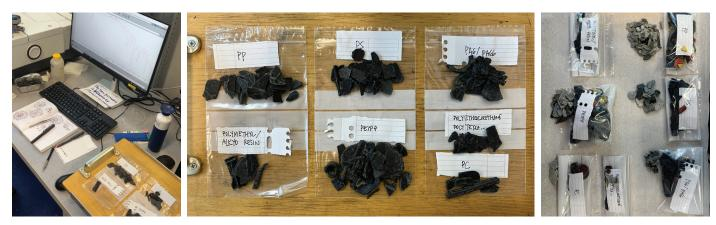
Appendix.15 FT-IR identification process after manual colour sorting (1) FT-IR setup, (2) placement of plastic shreds to respective polymer category of SDA-2, (3) placement of plastics shreds of SDA-1
