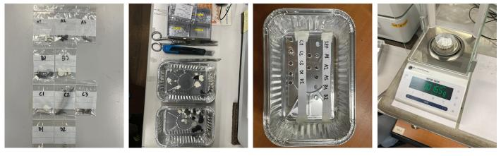
Appendix.6 DSC preparation (1) sample selection, (2) cutting samples, (3) sealing them inside a sample pan, (4) weight collection of each sample
