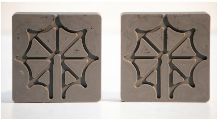
Figure 77: Final ABS-like resin printed mould used for the injection molding Spacer 10 (Source: Author)
