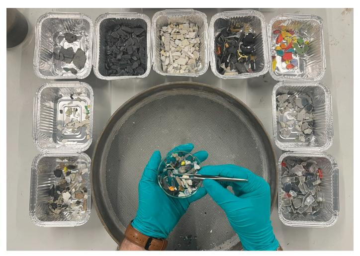
Figure 50: The manual colour sorting setup based on physical characteristics (Source: Author)
