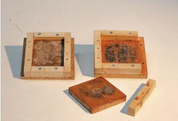
Figure 53: The detachable wood moulds 100 x 100 x 4 mm (see left) and 80 x 100 x 4 mm (see right) (Source: Author)
