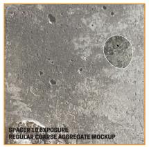
Figure 96: The contact point exposure inspection of Spacer 10 (Source: Author)
