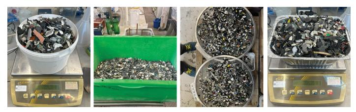
Appendix.3 Large-scale water separation steps (1)input weight, (2)density bath, (3) sink/floating fraction, (4) weighing floating fractions before drying
