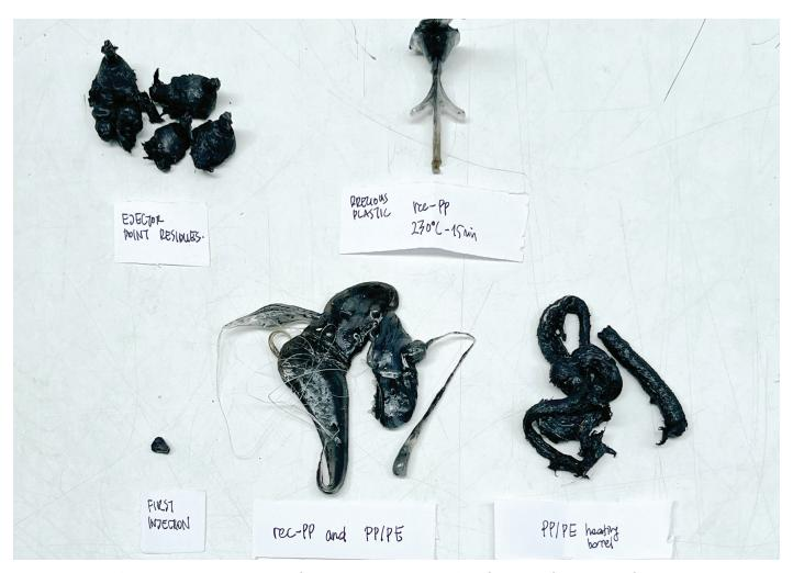
Appendix.21 Collected residues from the injection molding from the failed trials for Spacer 10
