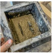
Figure 94: Mould preparation steps (1) Fixing the rebar and snapping the spacers (2) Pouring the design mix(3) Vibration table (4) Leaving the mould to cure (Source: Author)
