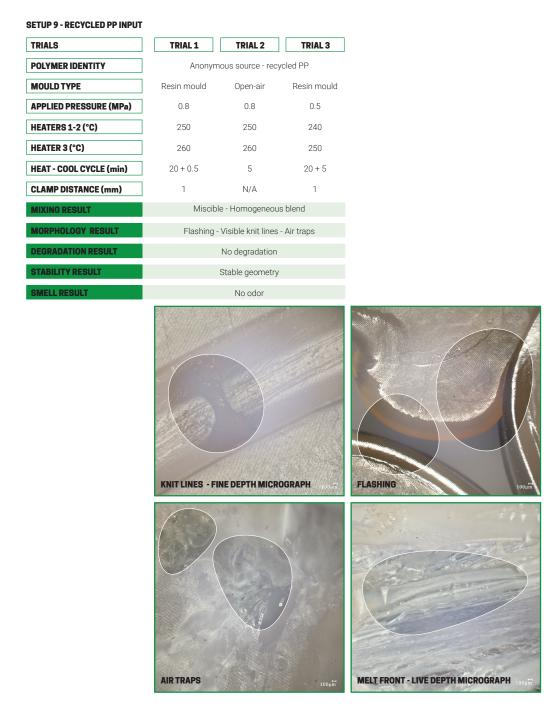
Table 18: Ninth setup with pneumatic plunger-type injection molding with rec-PP input (Source: Author)
