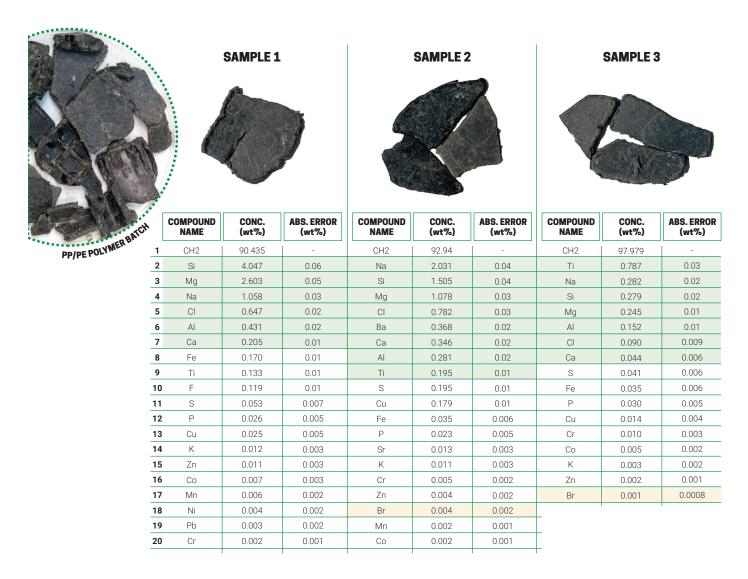
Table 9: XRF results for the three samples with inidication of contaminants (green) and Bromine (orange) (Adaped from: Ruud Hendrikx)
