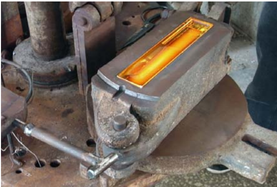
Fig.87 The casting process. The blocks were produced in moulds with high accuracy and controlled cooling process to avoid residual stresses.
