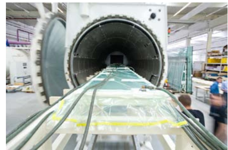
Fig.126_ Vacuum Bag lamination in large autoclaves. Photo courtesy of Seele Sedak GmbH.
