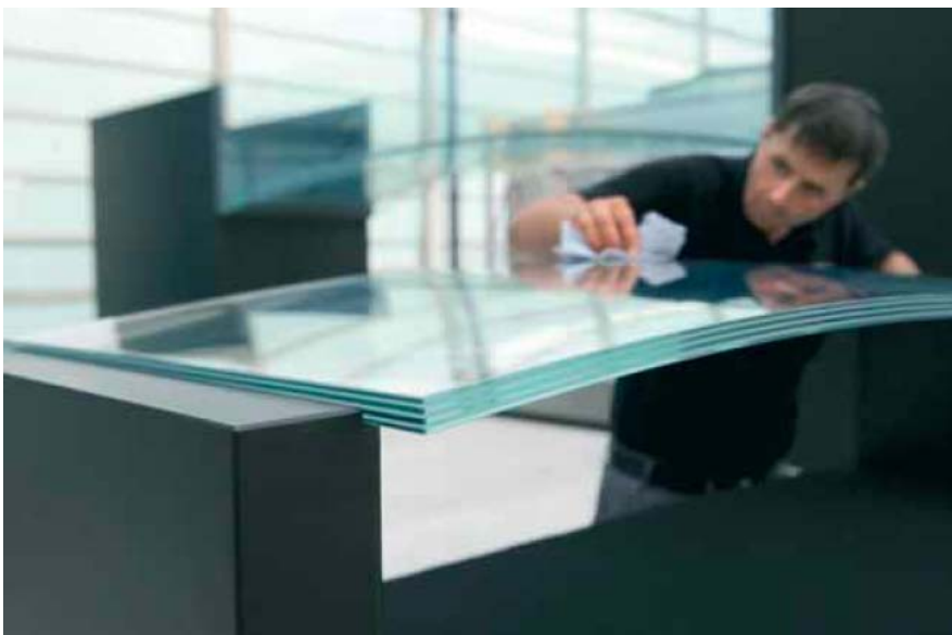
Fig.76_ Cold bending lamination process. Courtesy of Seele Sedak
