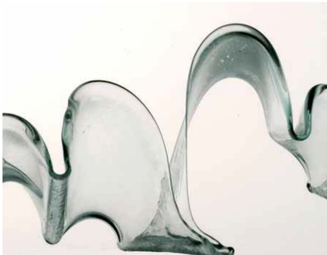
Fig.98_ Deformed glass plane ( Linear supports ). < www.glassfiles.com >
