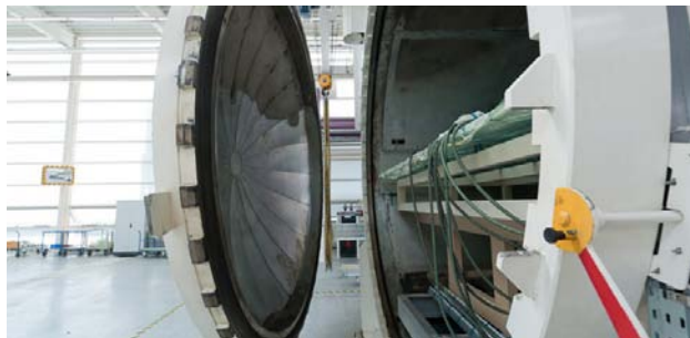
Fig.125_ The largest lamination autoclaves. Photo courtesy of Seele Sedak GmbH.
