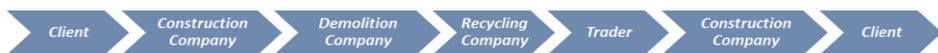
Figure 1-10 : Different steps of transferring the ownership of EOL concrete in the conventional concrete recycling business.
