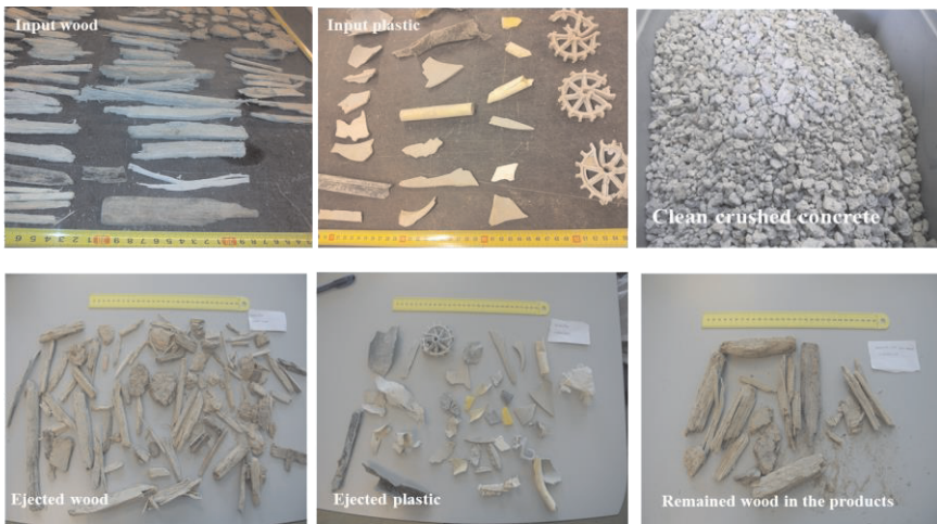
Figure 6-11: Input of wind sifter (upper images) which consists of wood, plastic and clean +16 mm crushed concrete. Images at the bottom demonstrate the removed wood and plastic using wind sifter and remained wood in the products.
