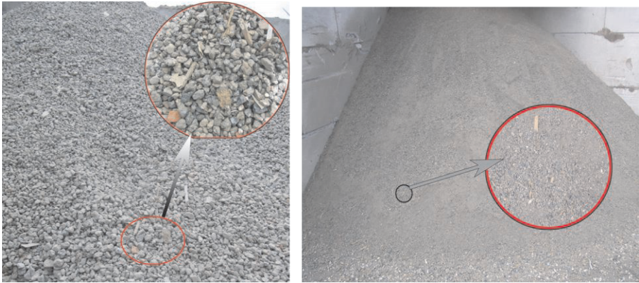
Figure 6-7: Left) +16mm RA which still contain contaminants, Right) ADR fines in which light contaminants like wood and foam are concentrated.
