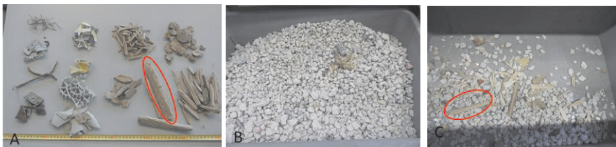
A: Example of input contaminants to the NIR sensor sorter, B: Accepted materials (NIR sensor sorting out put), C: Ejected materials (NIR sensor sorting out put)
