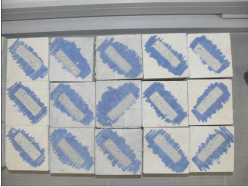
Figure 3-19: Concrete samples after the abrasion resistance test.
