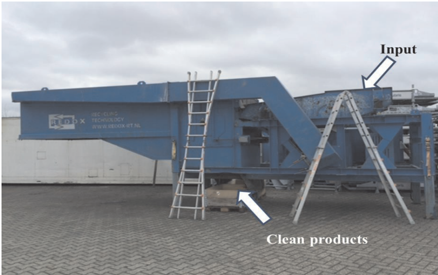
Figure 6-10: Wind sifting facility in REDOX.
