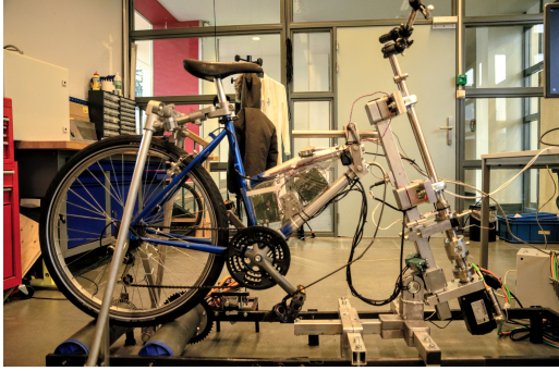
Figure 1: Delft fixed base bicycle simulator with model based haptic feedback torque
