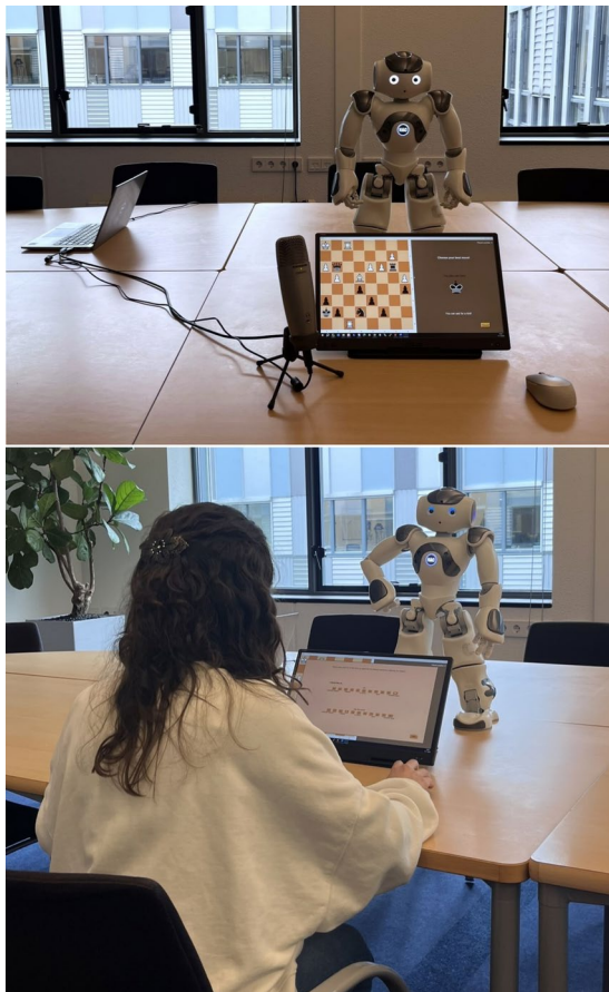
Fig. 7 Experimental setup: The participant sat at a table in the room. The Nao robot was placed on top of that table, facing the participant. A display was placed on the table between Nao and the participant. The display showed the chess puzzles and the questions asked to the participant during the session. A mouse and a microphone were placed on the sides of the display. The microphone and the display were both connected to a laptop that managed the HSRI and that was connected via Wi-Fi to Nao to steer its behavior via Python
