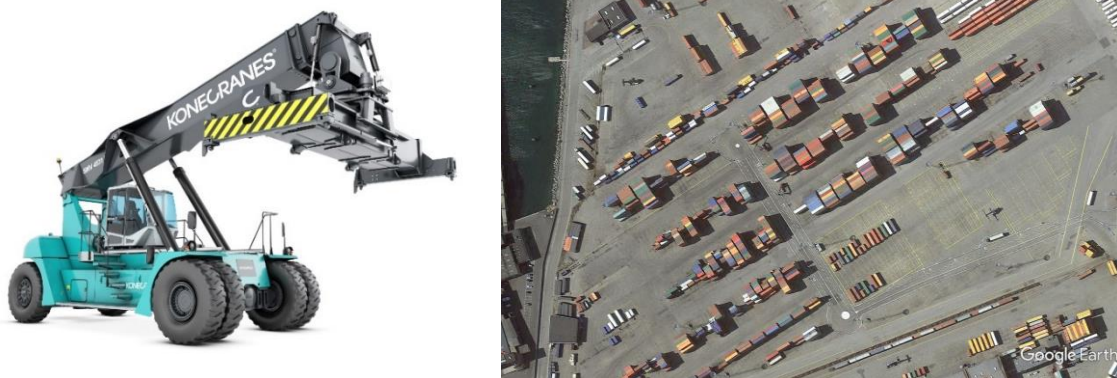
Figure 13 Reach Stacker and Container Terminal using Reach Stacker in Port of Aarhus, Denmark (Kone Cranes, 2020f), (Google Earth, 2018c)
