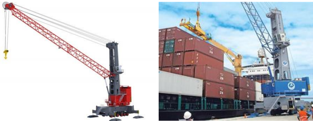
Figure 9 Mobile Harbor Crane and Container Terminal using Straddle Carrier in Port of Paramaribo, Suriname (Kone Cranes, 2020b), ( https://www.forkliftaction.com/news/newsdisplay.aspx?nwid=8272 )
