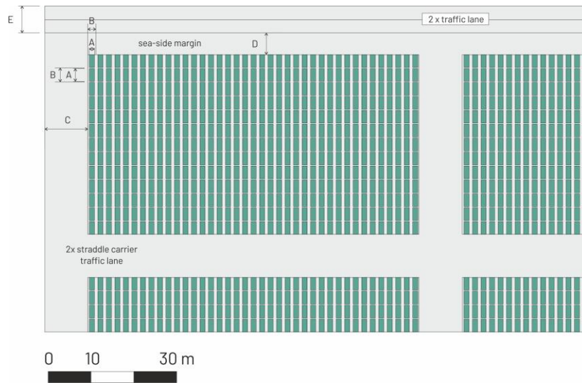
Figure 54 Illustration of the design rules applied for yard area (SC) (Author's Illustration)
