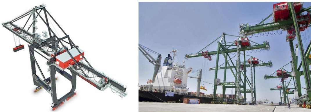
Figure 8 STS Crane and Container Terminal using Straddle Carrier in Port of Teluk Lamong, Indonesia (Kone Cranes, 2020a), ( https://www.nauticexpo.com/prod/konecranes/product-30447-189113.html )
