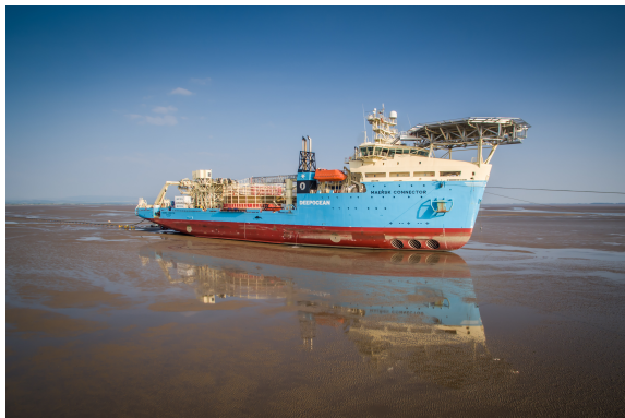
(c) Beached Shallow Water cable lay vessel (Navingo [97])
