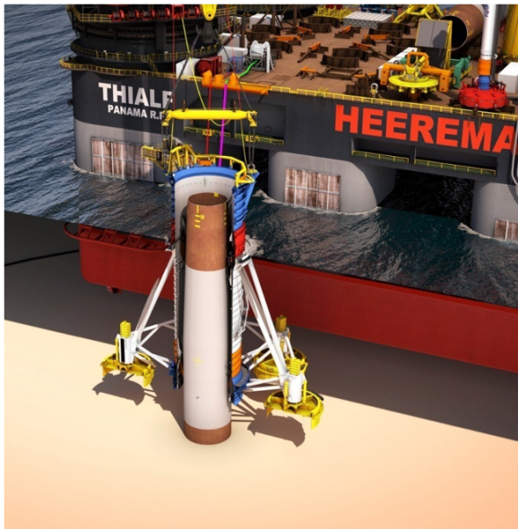
Figure 1.2: Rendered image of the T-NMS 10000 installed around a MP during deployment (IQIP, 2023).
