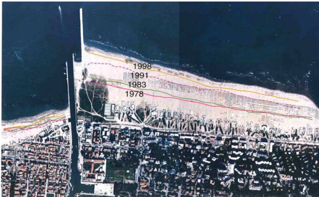
Fig. 2.35. Evolution of the coastline of Lido degli Estensi from 1978 to 1998 (fount Arpa 2002)
