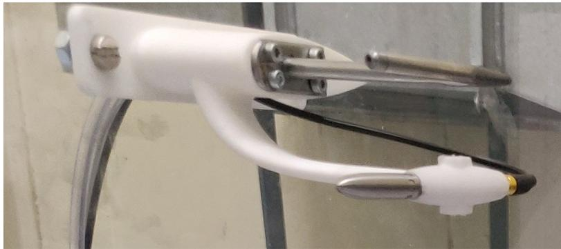
**Figure 5.9:** Freestream microphone and pitot tube setup
