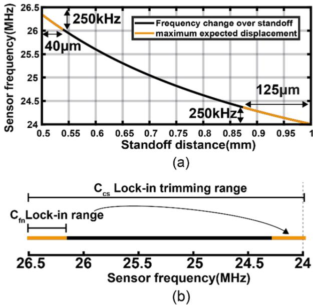
Fig. 5. Frequency profile of the free-running sensor oscillator with (a) fixed tank's capacitance and (b) employing  $C_{cs}$  switched capacitor banks to trim the oscillator center frequency to the desired 24 MHz for different standoff distances.
