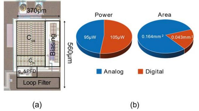
Fig. 12. (a) Micrograph of the EC sensor interface. (b) Power and area breakdown.
