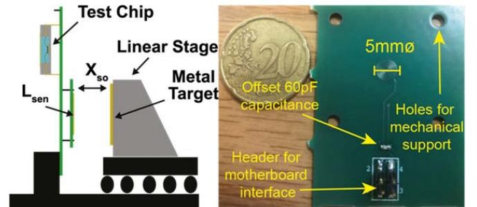
Fig. 13. (a) Measurement setup. (b) Sensing coil.
