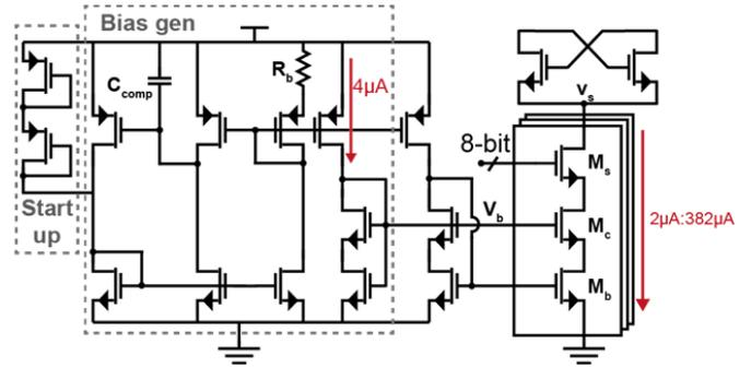
Fig. 9. Current DAC implementation along with bias generator.
